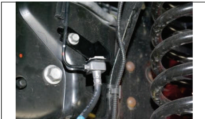
Reinstall block into bracket with retaining clip.
