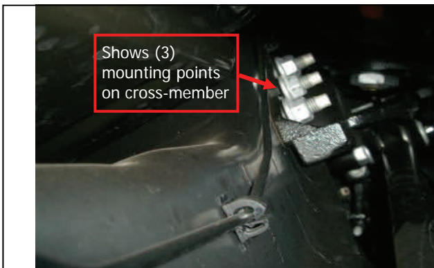
Shows (3) mounting points on cross-member Install new bracket with factory hardware and torque to spec.
