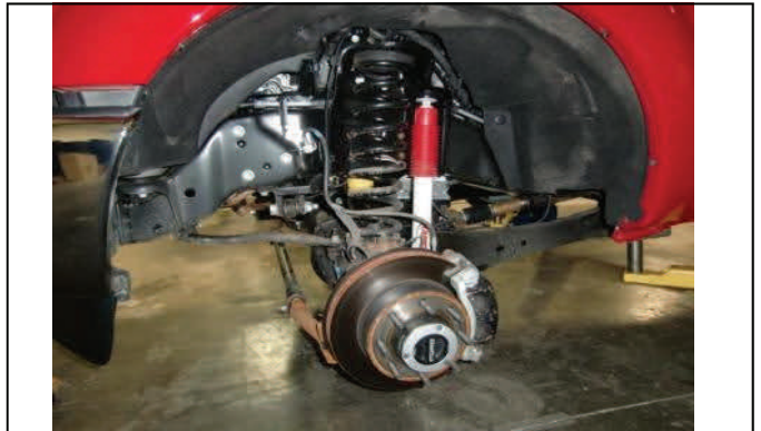
Remove front wheels and tires.
