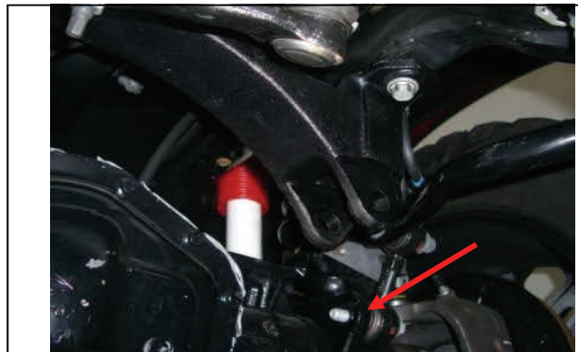
(.05-10) Re-attach and tighten sway bar end links.
