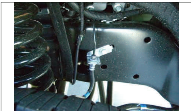
(08-10) models require drilling new 3/8 hole below OE hole.
