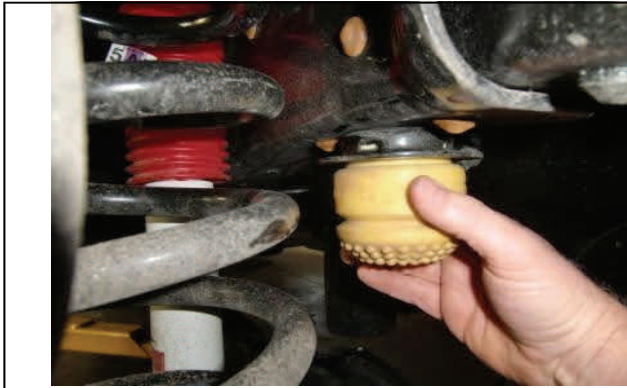
Remove bump stop and unbolt bracket from frame.
