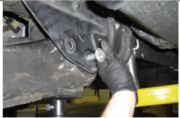
Support radius arm and remove attachment bolts
