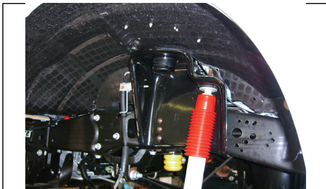
Carefully lower front axle and remove front coil springs.
