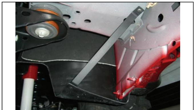
(05-10) Install fender liner strap to clear larger wheel/tires
