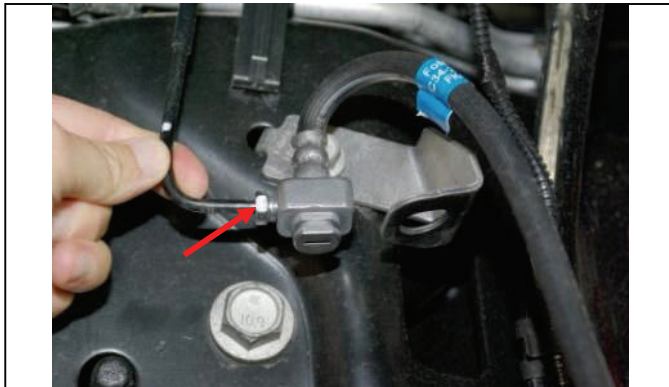
Loosen hard line ferrule rotate block 180 degrees and tighten
