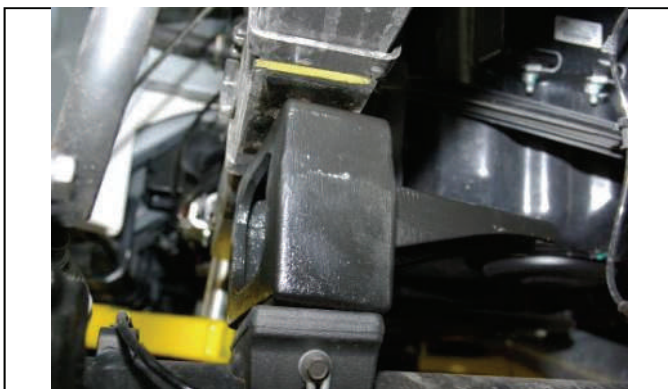
Lower axle enough to install taller block, align and raise axle
