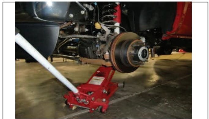
Support front axle with floor jack(s).
