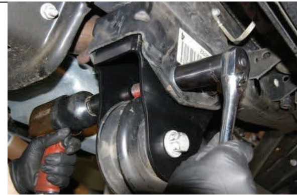
Tighten hardware and leave OE bolt loose until on ground.
