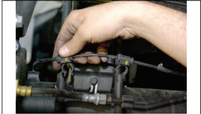
Vehicles with ABS/TC remove clips from U-bolts.
