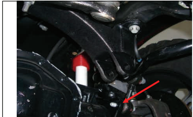
(.05-10) Re-attach and tighten sway bar end links.
