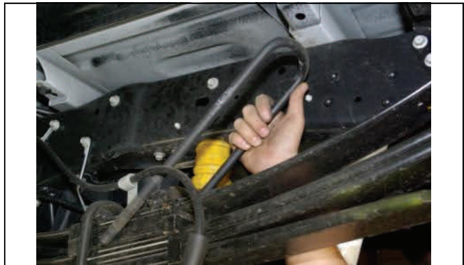
Remove U-bolts and slowly lower axle to remove OE block.
