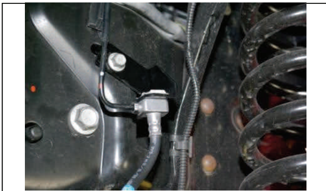
Reinstall block into bracket with retaining clip.
