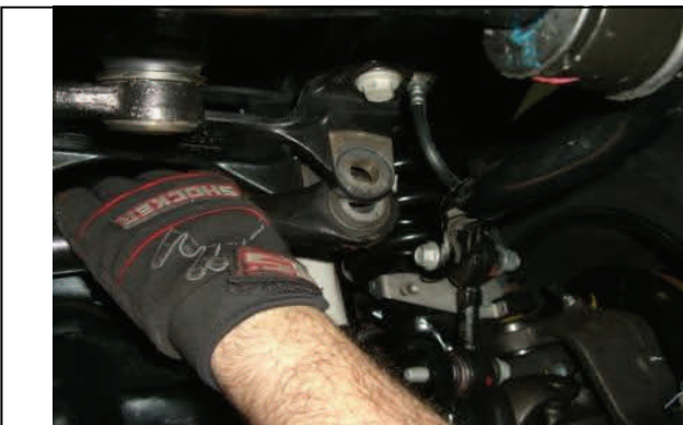
Re-attach trac bar to frame mount and torque to spec.
