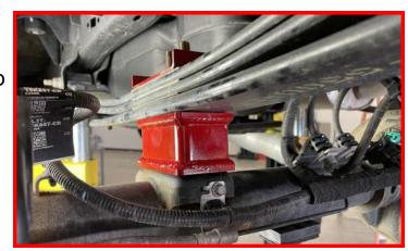
Install the provided u-bolts, and nuts. Snug the u-bolt nuts but do not fully tighten at this time.
