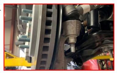
Install the sway bar end link into the knuckle using the factory hardware.
