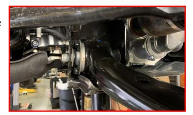
Install the supplied alignment cam plate over pivot bolt so pin fits in existing small hole in frame and then install alignment eccentric cam nut by threading bolt into nut.
