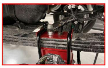
Install the shock extension using the provided M12 bolts, washers, and nuts to the top of the factory shock.
