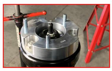
NOTE: IF INSTALLING KIT ON A VEHICLE EQUIPPED WITH AUTO ADJUSTING HEADLIGHTS OR CCD, REMOVE THE BALL STUD MOUNTED TO THE FACTORY CONTROL ARM BRACKET. RETAIN THE MOUNTING HARDWARE.
