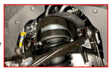
Install the ball joint boot spacer between the bottom of the boot and the top of the knuckle and raise the knuckle high enough to install the ball joint into the knuckle.
