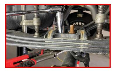
Remove the factory u-bolt retainer plate.
