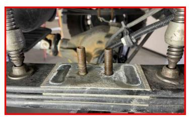
Install the supplied u-bolt retainer plate, Using the factory center pins.
