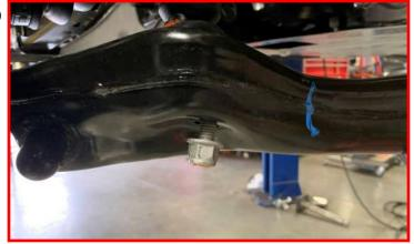
Using an appropriate jack, carefully jack the lower control arm into the frame side pivot pockets. Install the factory pivot bolts.
