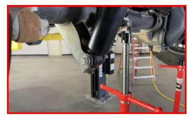
Remove the rear sensor bracket from the forward axle center pin.
