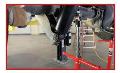
Prior to installing wheels, complete all installation steps on the opposite side. Install the wheels and lower the vehicle to the ground. Torque the lug nuts to the wheel manufacturers specs. Jounce the vehicle to settle the suspension to the new ride height. Torque the lower control arm hardware to 200 ft-lbs, u-bolts to 110-ft/lbs and all shock hardware to 75-ft/lbs.
