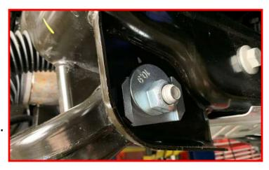
Tighten the top strut nuts.
