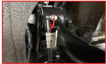
Using the supplied M10 nuts, install the completed strut assembly into the frame 180 degrees from the original orientation making sure that the offset of the top spacer is going in towards the frame and that the stamped word "OUT" on the spacer is going towards the outside of the vehicle. Do not tighten at this time.
