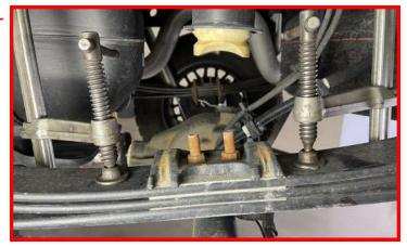
With the leaf pack clamped, remove the center pins.
