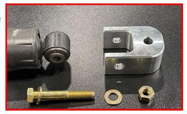
Install the shock into the frame using factory hardware. Ensure you are installing with the extension up.
