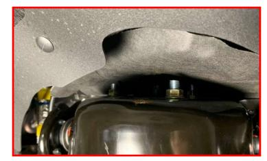
Carefully route the CCD solenoid harness over the tie rod.
