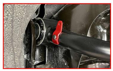
Install the front sensor ball stud into the upper control arm clamp using the factory hardware.
