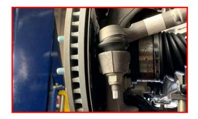
Loosen but do not remove the top strut nuts.
