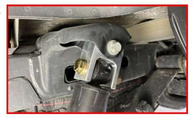
Install the lower shock to the axle using factory hardware.
