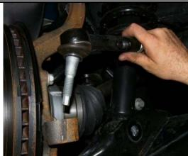
3) Loosen but do not remove the upper ball joint nut. Break the upper ball joint loose from the steering knuckle. DO NOT REMOVE THE UPPER BALL JOINT NUT.
