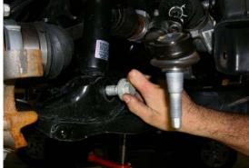
5) Remove the two lower control arm mounting bolts. Use a jack to support the lower control arm and take pressure off the bolts during removal. Below: Remove the three upper strut mounting nuts. Push the lower control arm down a little and remove the strut.
