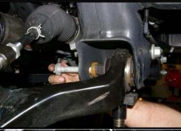
10) Tighten the upper ball joint. Torque to factory specs. Tighten the three upper strut mounting nuts, reinstall the tie rod end, and tighten the lower strut mounting nut. Install the two 10mm brakeline support bolts. Install ABS line back into the brake line support.
