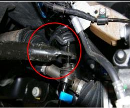
9) Install the two lower control arm bolts but do not tighten.
