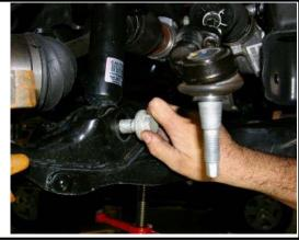
8) Make sure the upper sway bar end link gets reinstalled at this time. Torque to factory specs.
