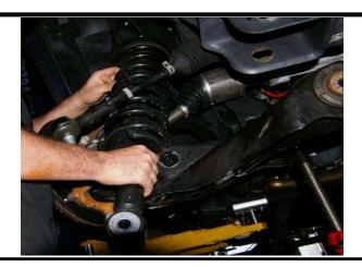
6) Reinstall the strut onto truck. Be sure to leave the upper strut mounting nuts loose so that the strut can still be maneuvered when installing the lower mount.
