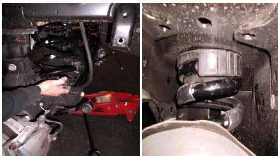
27. Reinstall the coil spring with the spacer.
