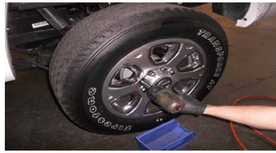
30. Reinstall the rear wheels.
