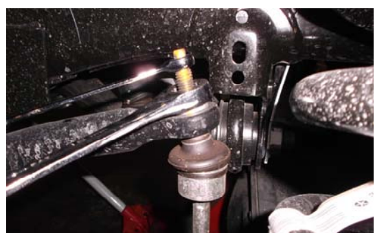
4. While front axle is supported, remove the sway bar end links.
