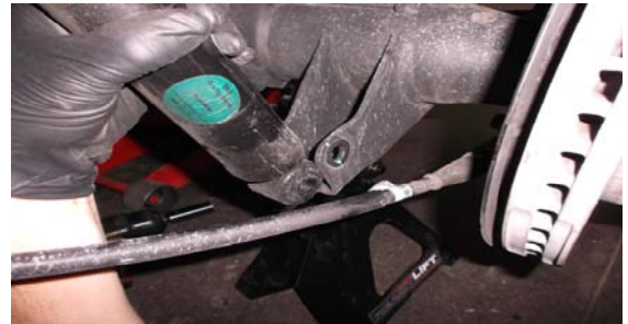
24. With the axle supported, unbolt the shocks from the axle.
