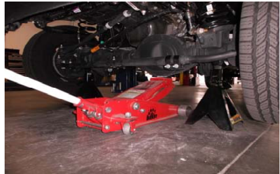
2. Lift the front of vehicle by the frame, then support the axle.
