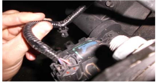
6. Unhook the wheel speed sensor wire line from the mount on the passengers side of the axle.
