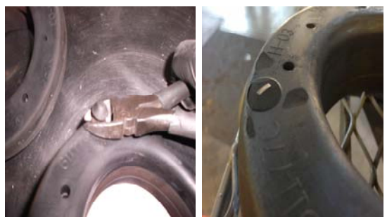
12. On OE spring isolator, cut off the rubber locating tab.
