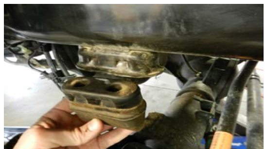
10. Remove the factory bump stops from the frame.
