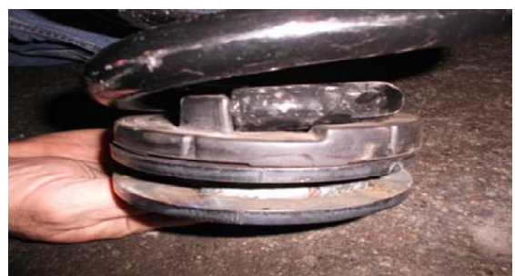
26. Place the coil spacer under the lower spring isolator.
