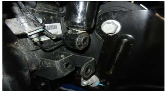
8. Unbolt the front shocks from the axle. Leave the tops bolted.
