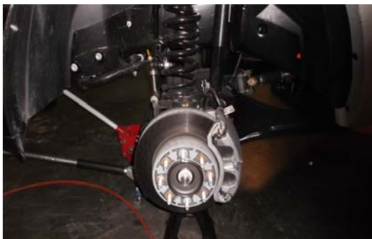
3. Remove the front wheels.
