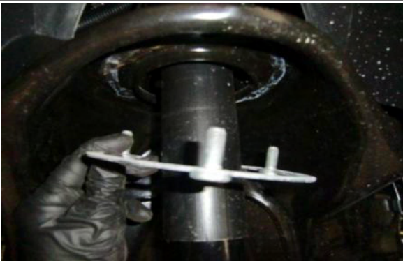
Remove factory retainer plate & nuts.
