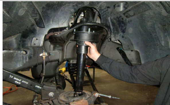
Install ReadyLIFT Coil Spacer
