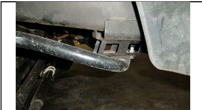
Install Sway bar drops. "off setting bar to the rear of vehicle"
