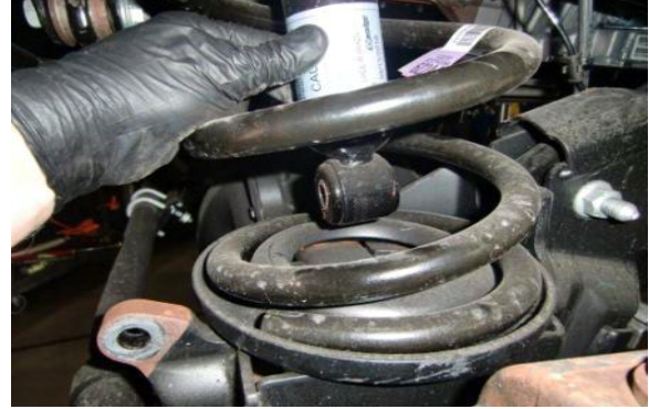
Slowly lower axle to remove tension on coil spring.
