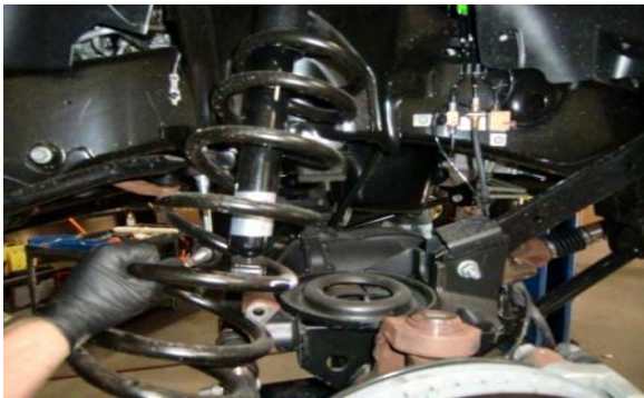
Remove spring towards the front of vehicle.
