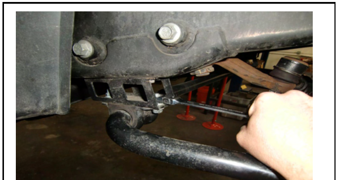
Tighten drop down bracket and sway bar.
