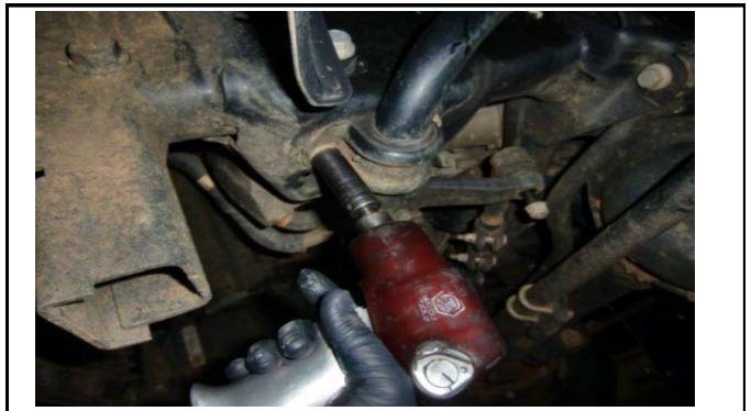
Disconnect sway bar from frame.
