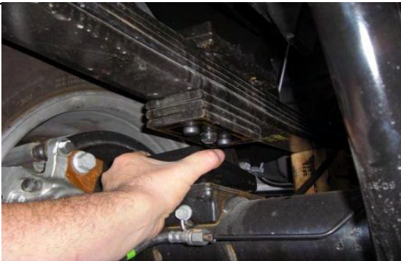
Place new lift block on axle pad, center pin down.
