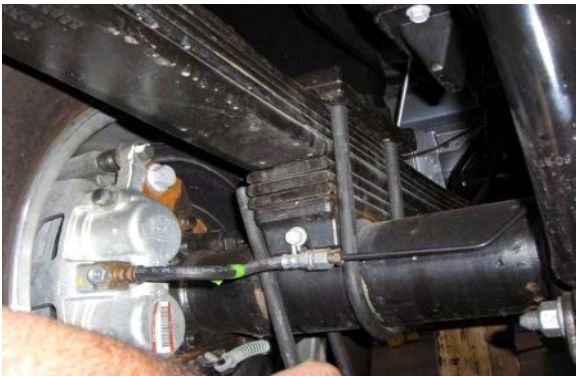
Disconnect U-bolts and remove, one side of vehicle at a time.
