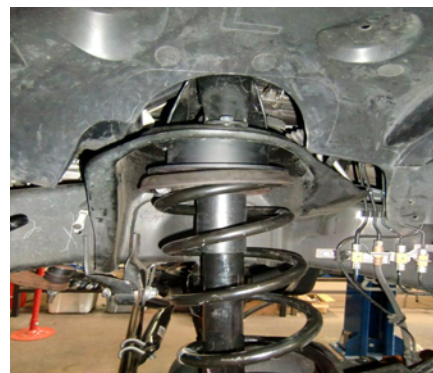
Re install Isolator and coil spring
