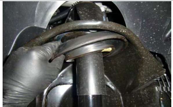
Remove Spring isolator if it did not come out with Coil Spring
