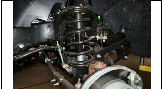
Picture of Front suspension. Support Front axle with jack.
