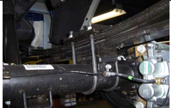
Support axle and disconnect lower shock mounting hardware.
