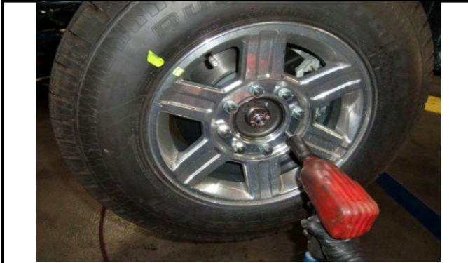
Raise front end of vehicle, support frame and remove wheels
