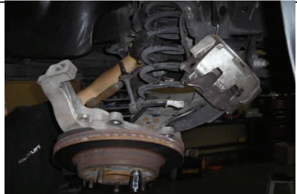
Slowly lower suspension and remove coil spring.
