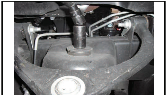
Disconnect upper shock mount and bushing
