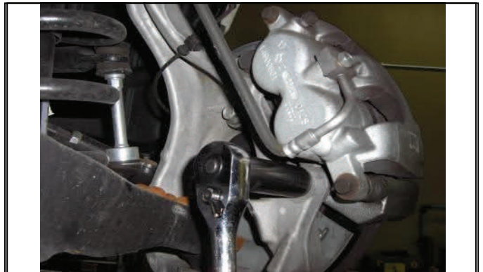
Remove brake calipers
