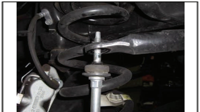
Disconnect upper sway bar end links and bushings
