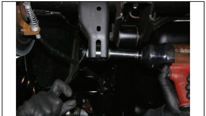
Remove lower shock mounting hardware.
