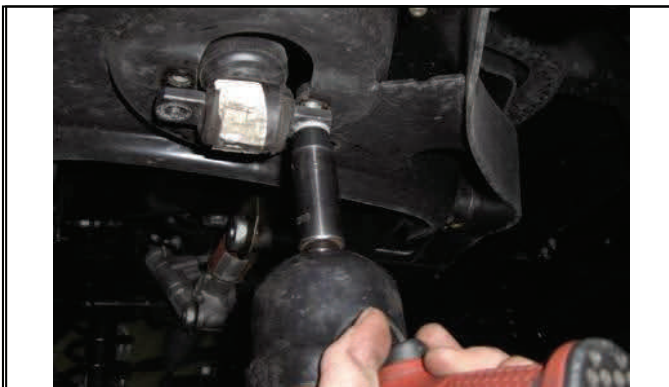
Disconnect lower shock mounting bolts.
