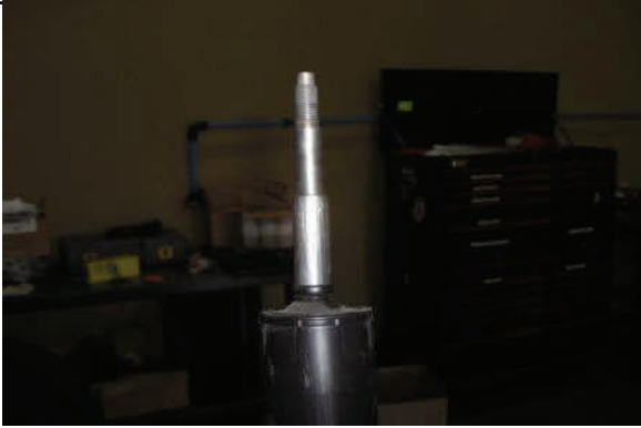
Install and tighten new upper shock extension
