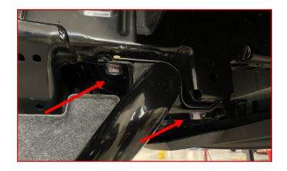
Torque the sway bar end link factory hardware to 80 ft-lbs.
