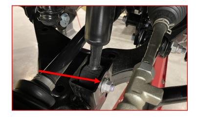
Remove the four (4) upper strut bolts.
