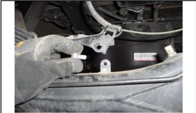
Disconnect ABS wiring brackets from axle.
