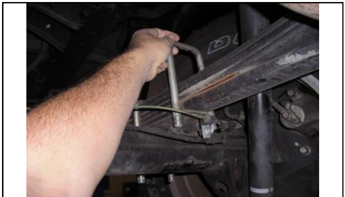
Carefully lower axle and remove u-bolts
