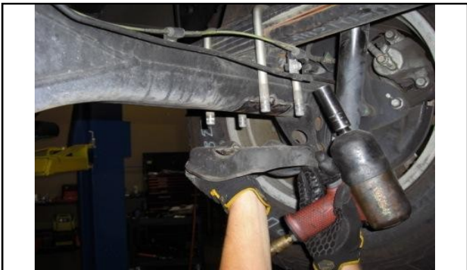
Remove u-bolt nuts and lower plate.
