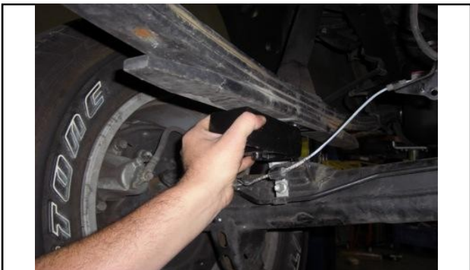
Place new lift block into position between axle and leaf pack.
