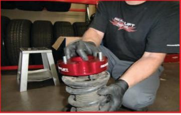
Raise the LCA, reconnect the strut to the lower control arm using the factory hardware. Do not tighten at this time.
