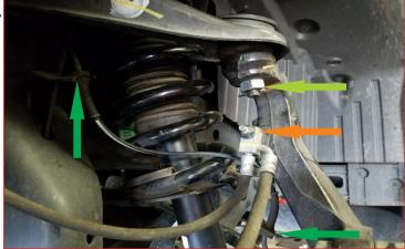
Remove the three upper strut mounting nuts.
