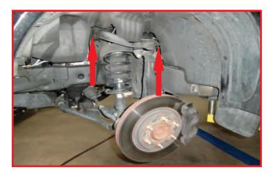
Remove ABS wire from their steel brackets. Remove the brake lines from the knuckle. Remove the cotter pin from the upper ball joint, and loosen but don not remove the ball joint nut.
