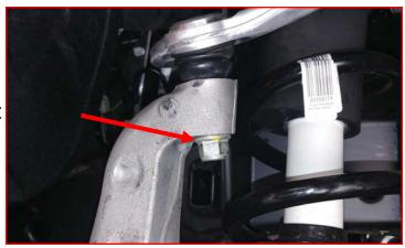
Support the lower control arm with a suitable jack. Remove the lower strut mounting bolt from the lower control arm. Retain the factory bolts.
