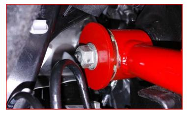
Once upper control arms have been properly torqued, install the supplied top strut spacer on the top of the strut assembly. Install completed strut assembly into the vehicle using the supplied M10 serrated flange nuts.
