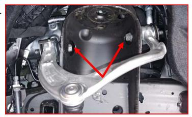
Ensure you have the proper replacement control arm, they are side specific and need to be installed on the correct side.
