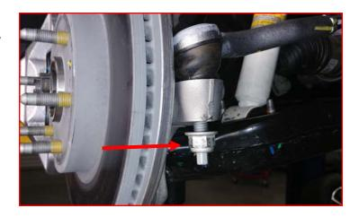
Remove the ABS sensor harness and the brake-line bracket from the knuckle and hang out of the way. Retain factory hardware.
