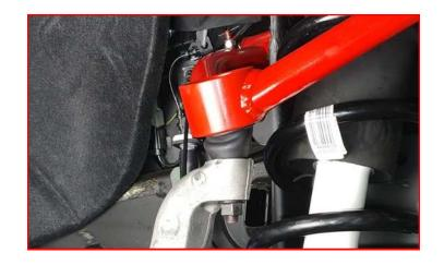
Install the sway bar drop link into the lower control arm using the factory nut.
