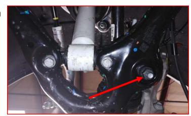
Remove the CV axle nut. Press axle back through hub to allow for greater misalignment and ease in the removal/installation process.
