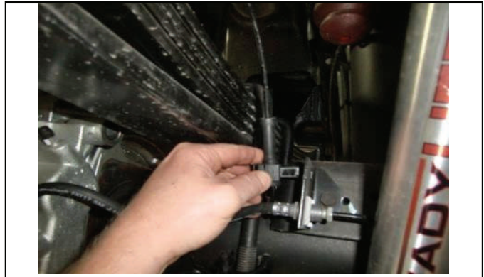
Release ABS clip from bracket on axle.
