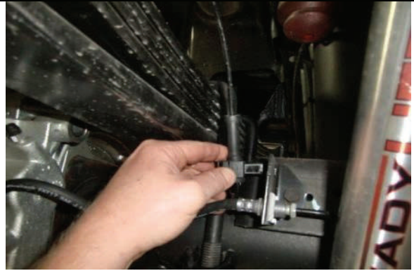
Release ABS clip from bracket on axle.
