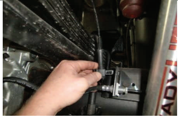
Release ABS clip from bracket on axle.
