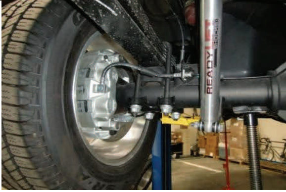
Raise and support vehicle on level ground and support frame.
