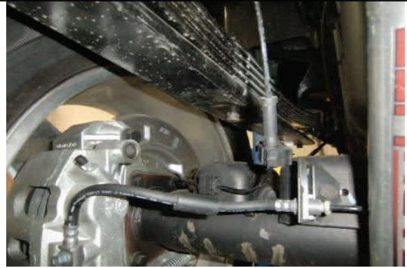
Remove U-bolts and lower axle to allow lift block positioning
