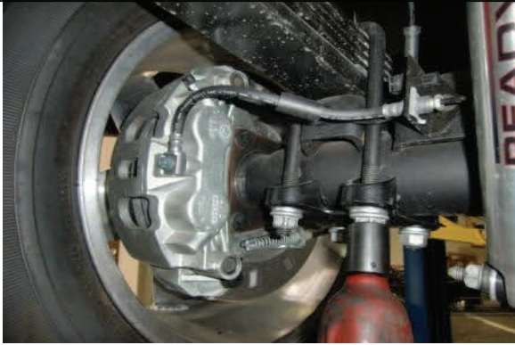
Support axle and remove U-bolt hardware and axle bracket
