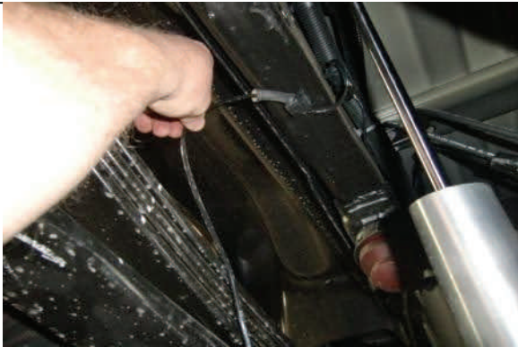
Slide ABS wire clip at frame up to gain slack to avoid damage
