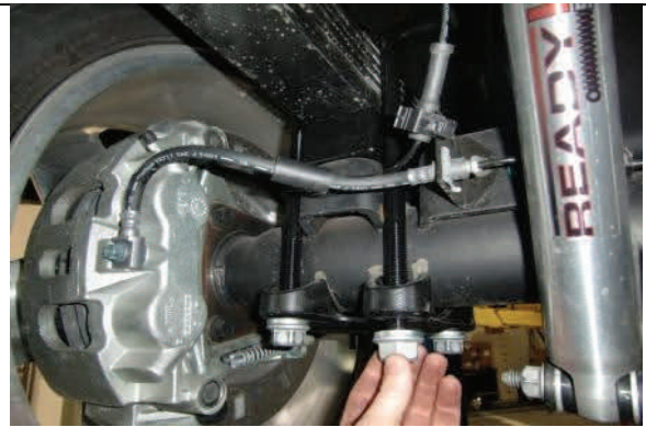
Raise axle aligning center pin and install new U-bolts/nuts.
