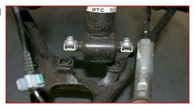
Remove the upper strut mount at the frame.
