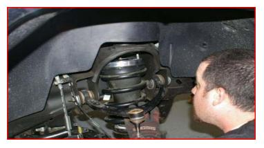
Raise the lower control arm and install the ReadyLIFT lower strut extension using the factory hardware. Torque to 45 ft-lbs.
