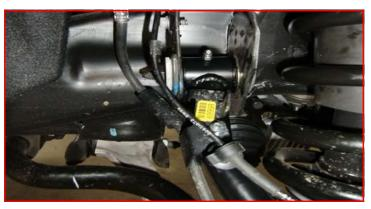
Attach the ABS wire to the frame rail with the factory clip. Re-connect the electrical connector.
