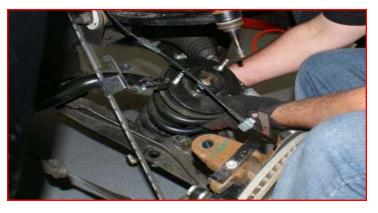
Remove the upper control arms. Make sure to note the orientation of the alignment cams for re-installation later.
