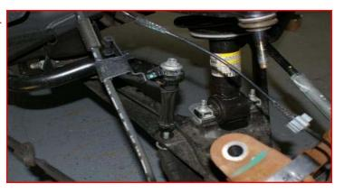
Attach the upper ball joint to the knuckle using the provided hardware (4wd guide the CV axle through the hub bearing while installing the upper ball joint). Torque to 85 ft-lbs. DO NOT use an impact.
