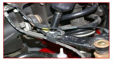
Remove the sway bar end links from the sway bar and lower control arm.
