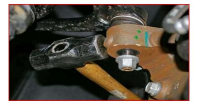
Remove the lower strut from the lower control arm.
