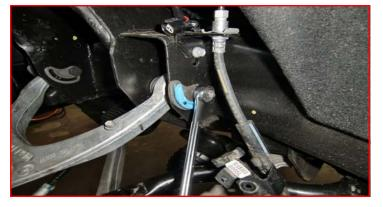
Install the appropriate side ReadyLIFT upper control arms into the frame using the previously removed cam bolts and cams. (New design control arms do not have Zerk fittings and do not require grease) Do not tighten at this time.
