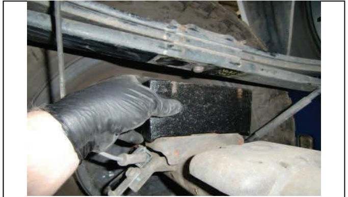
Shown (3.0" block) replacing factory block on 4WD models
