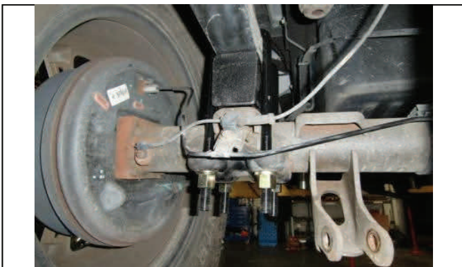
Tighten hardware and reinstall lower shock into mount
