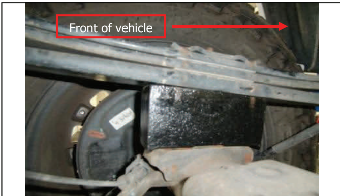
Raise axle and center locating pin on leaf pack. Note: taper
