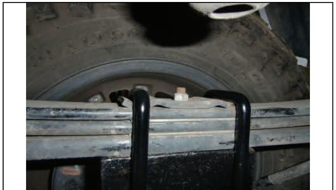
Place u-bolts over saddle on leaf pack and over axle
