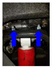
Measure and record the torsion key adjuster bolt length and part number. Remove the torsion bar adjustment bolt.
