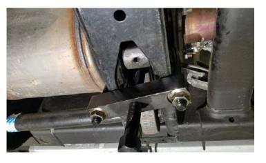
Install the differential skid plate with the rear mount only at this time. Use supplied M10x35 bolts, M10 fender washers and 1/2'' spacer. Hand tighten only.
