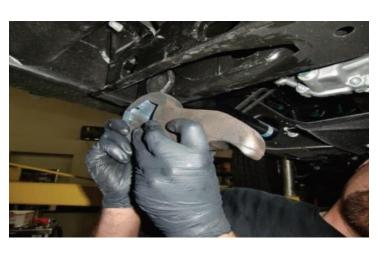
Install the ReadyLIFT keyway into the cross member while sliding the torsion bar into place. The tang of the keyway will be clocked slightly lower than the factory key. This accounts for the lift. Do not load the cross pin or bolt adjuster at this time. This will be done as one of the last steps.
