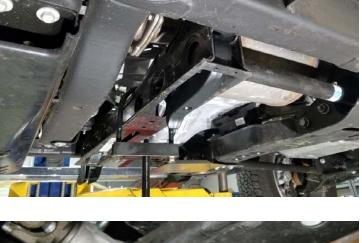
Loosen but do not remove the lower control arm bolts. This step is necessary to relax the bonded bushings for the new lift height. These bolts will be retighten when the kit is finished installed and the vehicle is on the ground.
