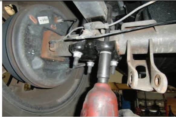
Remove u-bolt mounting hardware
