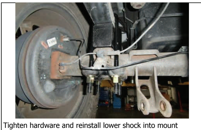
Reinstall axle mounting plate
