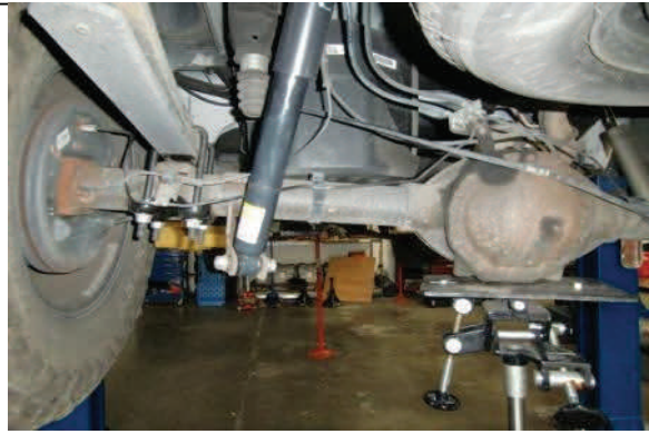
Support rear axle with jack
