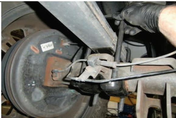
Remove u-bolts and axle mounting plate
