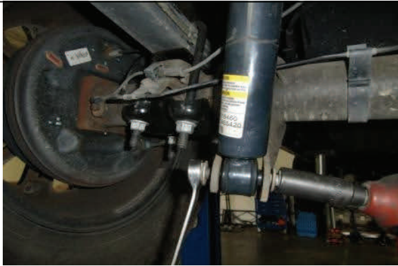
Disconnect lower shock from mount
