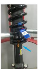
Compress the spring and shock, until the tension is released from the tension nut.
