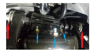
Remove ABS wire from the steering knuckle.
