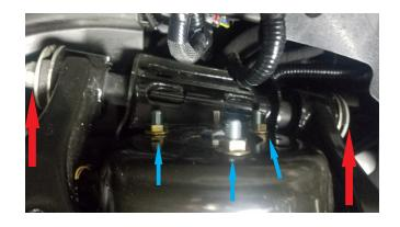
Remove ABS wire from the steering knuckle.
