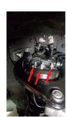
Using a jack raise the LCA and reinstall the bottom studs of the strut to the LCA hand tighten only.
