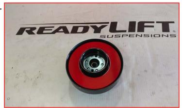
2.5" kit Pre-load spacer: Install the factory top hat onto the strut assembly 180 degrees from the factory orientation using the previous marks made as a guide. This is very important for spring to control arm clearances once the strut assembly is installed back into the vehicle.
