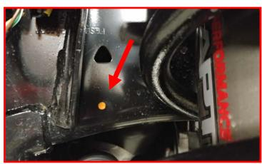
Route the coil over harness up along the control arm sensor harness on the frame rail and behind the plastic wheel liner using the factory clips along the way. Plug the electrical connector back in.
