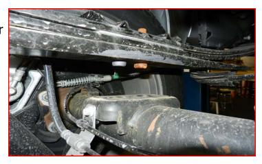
Locate the passenger side lift block, making sure the tapered end points to the front of the vehicle. Install the lift block on the axle pad aligning the pins. Raise the axle and the block up to the spring while aligning the center pins. Install the provided u-bolts, washers and nuts. Snug the U-bolt nuts but do not fully tighten at this time. Repeat steps for driver side. Lower the vehicle to the ground and torque the U-bolts to 110 ft-lbs.
