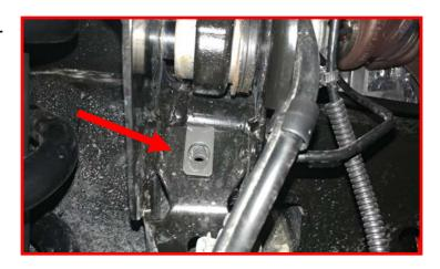
Install the ReadyLIFT provided urethane bump stop by screwing into the capture nut until fully seated.
