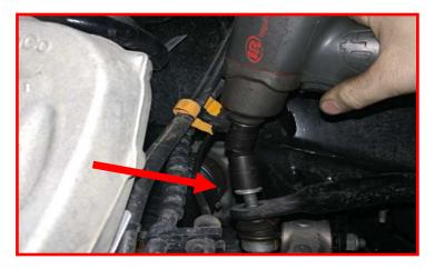
2019 and UP Models: Driver side, make a mark on the frame rail behind the coil over 1.25" back from the strut tower lip and 1.25" up from the bottom of the frame rail and use a 7/16" drill to make a hole. Paint all exposed metal with a quality rust preventative paint. Install the previously removed shock harness clip into the hole. Make sure to route the harness behind the coil over.
