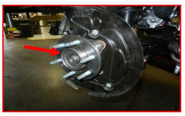
Jack the lower control arm up to add pressure to the strut. Putting a suitable jack stand at the rear of the vehicles frame will aid in keeping the load transfer from picking the front end up while jacking the lower control arm up.
