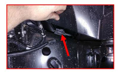
Driver side, locate the electrical harness on the coil over and follow it up onto the frame rail and into the engine bay. The wire follows the ABS harness.
