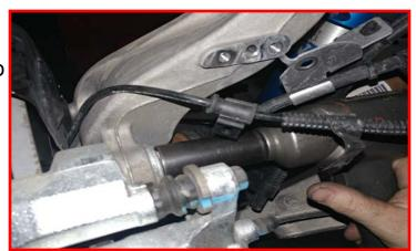
Install the outer tie rod end to the knuckle using factory hardware. Torque to 85 ft-lbs.
