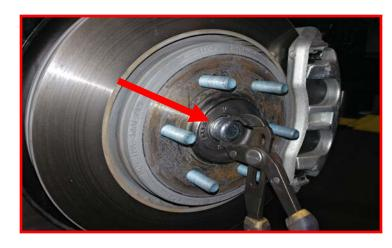
Remove the CV axle nut.
