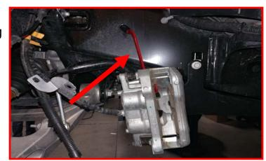
Loosen but do not remove the upper ball joint nut at the knuckle. Strike the ball joint boss with a dead blow hammer to dislodge the taper. Remove the ball joint from the knuckle. Support the knuckle as to not let it fall to protect the vacuum hub. Loosen but do not remove the upper control arm bolts at the frame rail.
