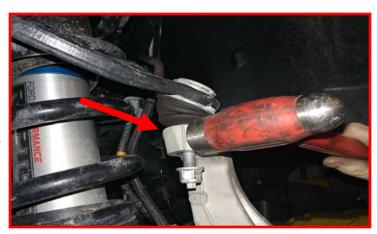
Support the lower control arm with a suitable jack. Loosen but do not remove the lower control arm bolts at the frame rail. Remove the lower coil over bolt.
