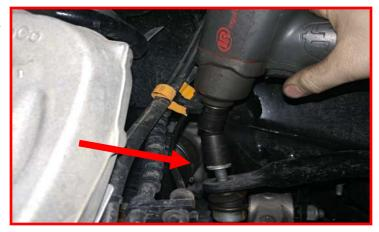
Remove the CV axle nut cover.
