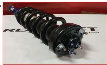
1.5" kit top extension only: If you are only installing the top extension kit, Put the strut assembly into a suitable spring compressor and release the tension. Rotate the factory top hat 180 degrees from the factory orientation using the previous marks made as a guide. Remove the strut from the compressor.
