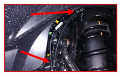
Mark another hole location in the plastic wheel liner in line with the original mounting hole but on the lower portion closest to the engine bay. Use a 7/16" drill bit and suitable drill to make the hole. Make sure to only drill through the plastic liner and not anything else. Move any wire harness that may be in the way to drill the hole. Install the coil over electrical connecter clip into the new hole.
