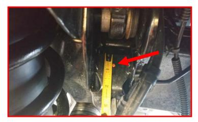
Drill out the mark with a 1/2" drill bit. Install the ReadyLIFT capture nut onto the frame.
