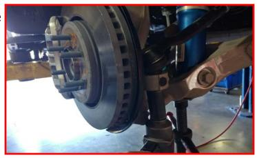
Install the brake line bracket to the knuck-le using factory hardware. Torque to 5 ft-lbs. Install the ABS line back to the frame, to the rubber brake line clamps, and knuckle using factory hardware. Torque to 165 in-lbs. Install the vacuum lines to the vacuum actuator.
