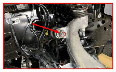
Remove the tie rod end on the knuckle. Retain the factory nut.
