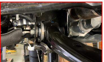
Tighten the top strut nuts.
