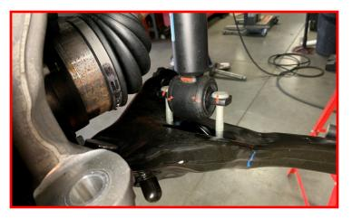
Continue to raise the lower control arm up until you are able to install the factory lower strut nuts.
