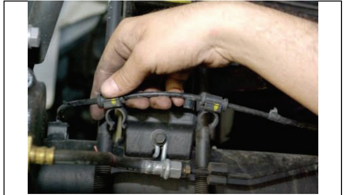
Vehicles with ABS/TC remove clips from U-bolts.
