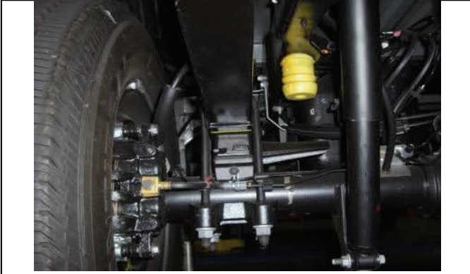
Raise Vehicle and support by frame. Support axle with jack.
