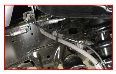
Install the metal brake line bracket to the frame rail using the factory hardware. Torque to 5 ft-lbs.
