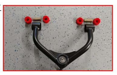
Install the ReadyLIFT appropriate side control arm to the frame rail using the factory hardware. Do not tighten at this time. To determine the correct side arm, there is a plugged hole on the back tube of the near the rearmost pivot.
