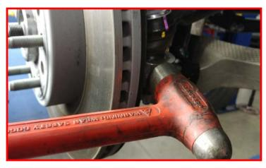
Remove the upper ball joint from the knuckle.
