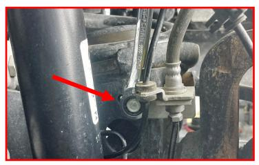
Remove the 18mm nut from the sway bar end link while holding the 8mm bolt so it does not spin.
