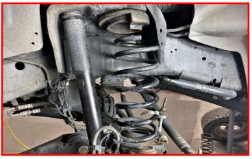
Remove the spring isolator and install the spring spacer with included hardware in the spring isolator locating hole.
