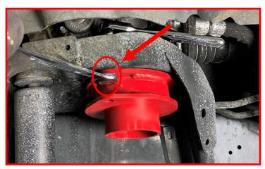
Place the spring isolator into the bottom locating hole on the spring spacer.
