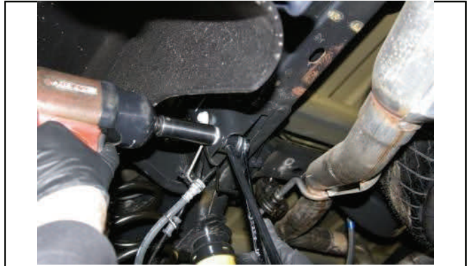
Disconnect upper sway bar end links.
