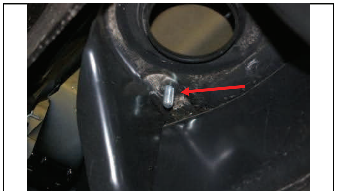
Use provided hardware to fasten new spacer and tighten.
