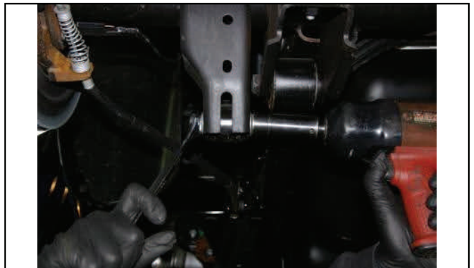
Remove lower shock mounting hardware.
