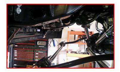
Lower the axle enough to remove the front springs. Install the ReadyLIFT ure-thane isolator, spring spacer, and then factory rubber isolator onto the spring. Raise the axle enough to hold the spring assembly in place.
