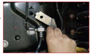
2017 - UP front brake line: Remove the brake line bracket at the frame. Remove the brake line bracket at the axle.
