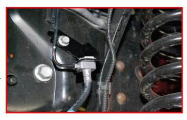
2017 - UP front brake line: Install the ReadyLIFT brake line bracket to the factory brake line using 5/16" x 3/4" bolts, washers, and nuts. Install the bolt facing outwards. Torque to 10 ft-lbs. Gently pull the metal brake line down while lining up the ReadyLIFT bracket to the original holes in the frame. Install using factory hardware. Torque to 5 ft-lbs.
