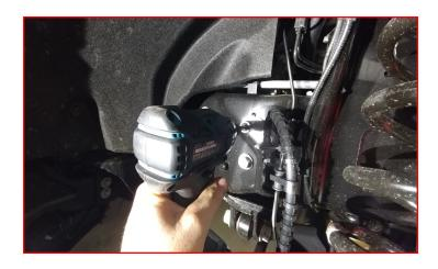
Remove the lower shock from the axle mount.
