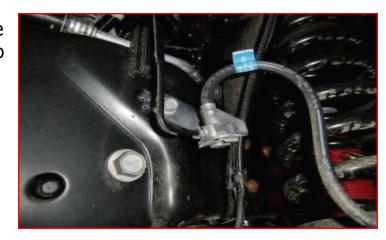
2011 - 2016 front brake line: Loosen the metal line ferrule nut at the rubber brake line block. Rotate the fitting down 180 degrees from factory and tighten. Remove the bracket from the frame.
