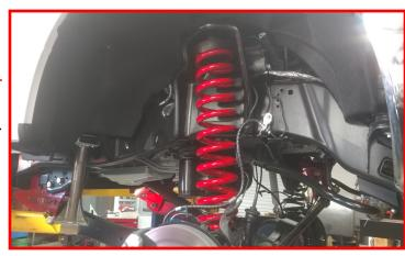
Install the ReadyLIFT sway bar drops to the frame using factory hardware. Torque to 35 ft-lbs. Install the sway bar to the ReadyLIFT sway bar drops using the 7/16" x 1 1/2" bolts, washers and nuts. Torque to 35 ft-lbs.
