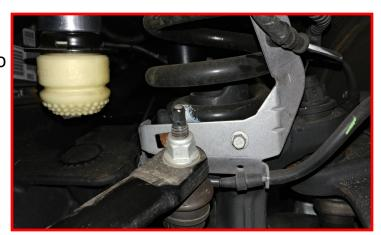
2011 - 2016 front brake line: Install the ReadyLIFT brake line drop bracket to the frame using the factory hardware. Torque to 5 ft-lbs. Note: The ReadyLIFT brackets look like the factory brackets except the locating flat is 180 degrees off. Install the brake line block using the factory clip. Reconnect the ABS line. Do not clip back to fender liner.
