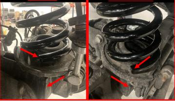
Install the front shock extension to the lower mount of the shock. Rotate the shock 90 degrees to allow for install to the axle mount.
