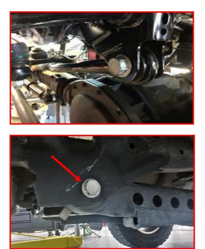
Loosen the rear radius arm bolt.
