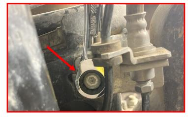
Reinstall the 13mm upper ABS and brake line bracket bolt located above the radius arm.
