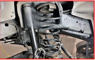
Retain the spring isolator and install the provided spring in the spring isolator locating hole.
