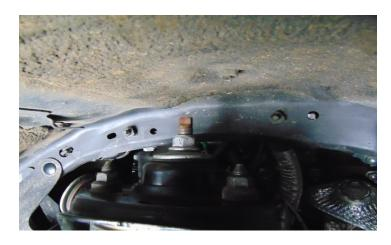
Add the lower strut extension to the strut assembly. Align the lower strut bushing with the through hole on the strut extension. Use factory hardware to fasten torque to 125 ft-lbs. Add the billet clamps to the strut extension use provided hardware torque 35 ft-lbs.
