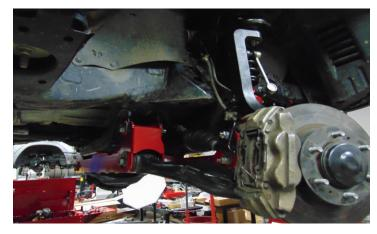
Install the OEM brake line bracket to the ReadyLift steering knuckle using factory hardware torque to 10 ft-lbs.
