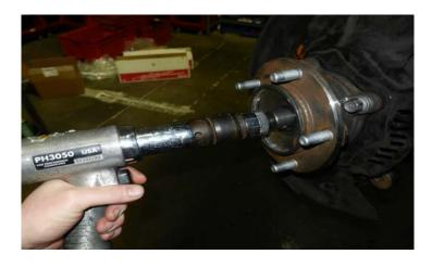
Remove the hub mounting bolts. Note: The bolts will not come off the hub.
