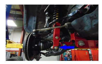
Protect the axle and ball joint boots with a wet rag or other suitable protection from grinding and welding sparks. Clean/grind off the paint/rust on the steering stop on the ball joint cradle. Weld the turn stop extension plates on their corresponding sides (match the contours of the stops) across the top and bottom.
