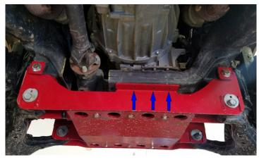
Install the ReadyLIFT skid plate. Use provided hardware, torque to 75 ft-lbs.
