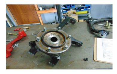
Reinstall the steering knuckle to the upper control arm use factory hardware torque to 67 ft-lbs then tighten until the castle nut aligns with the cotter pin hole, insert cotter pin. Place the axle in the knuckle bearing block. Raise the lower control arm and reattach the knuckle cradle to the knuckle. Use factory hardware Torque 180 ft-lbs with a drop of thread locker.
