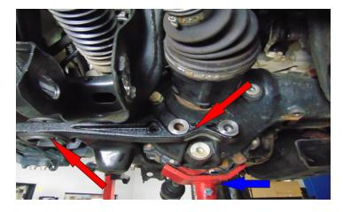
Install the new ReadyLift crossmembers use provided hardware, and cam block off plates. The cam block off plates have notches cut, start with the notches up you, can turn them 90 degrees for different fitments for frame deflection. Do not tighten hardware at this time.
