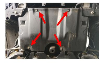
Remove the differential gravel guard.
