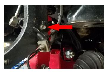
Install the ReadyLIFT front brake line extensions to the original brake line location on the frame using the factory hardware. Gently reposition the metal brake line to the extension fasten the brake line bracket to the extension using the provided hardware.
