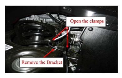
Remove the brake line from the frame and steering knuckle.
