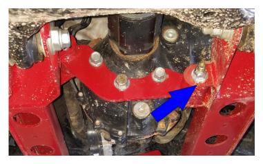
Reinstall the lower control arm to the ReadyLift crossmember use the original factory hardware. Do not tighten at this time.
