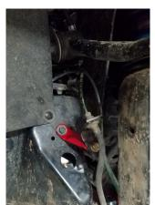
Install the wheel speed sensor to the ReadyLift steering knuckle. Use the factory hardware torque 5 ft-lbs.
