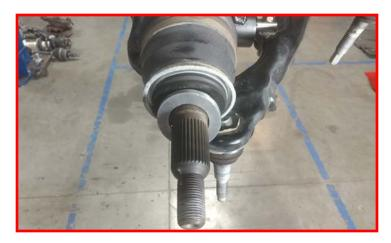
Install the completed ReadyLIFT knuckle assembly to the lower ball joint using the factory hardware while guiding the CV axle through the hub. Install the upper ball joint to the knuckle using the factory hardware if using the factory control arm and provided hardware if using the ReadyLIFT control arm. Torque the lower ball joint nut to 110 ft-lbs, and upper ball joint nut to 85 ft-lbs.
