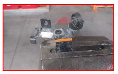
Locate the ReadyLIFT sway bar brackets. There is a left and right side specific. The mounting holes are offset to the front on the upper mount and to the rear on the lower. This locates the sway bar to the rear of the vehicle. Install using the factory hardware. Torque to 35 ft-lbs.
