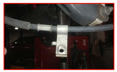
Remove the parking brake bracket in the driver side wheel well. Remove both cables from the bracket and let hang.
