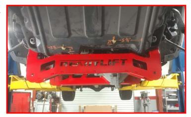
Make sure to re use the factory tapered washer that was under the nut. Make sure to install with the taper towards the frame rail. Do not tighten at this time.
