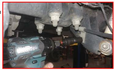
Open the mount up using a pair of pliers. Relocate to the cable behind the original keeper. Close the bracket back up. Reinstall to the shock mount using the factory hardware. Hand tighten only as this is a self tapped bolt hole and can strip easily.
