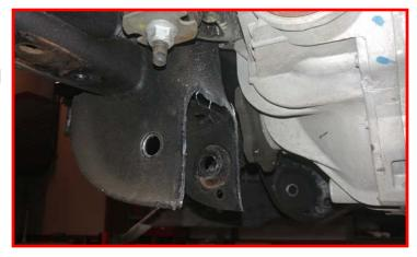
Support the front differential. Mark the front pinion to u joint for re-installation later. Remove the front drive shaft from the differential and let hang out of the way.
