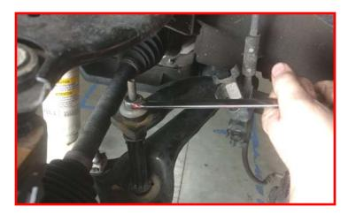
Loosen but do not remove the upper ball joint hardware. Strike the ball joint boss with a dead blow hammer to dislodge the taper.
