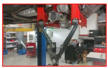
Install the CV axles to the differential using the factory hardware and a drop of thread locker. Torque to 35 ft-lbs.
