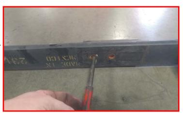
Locate the ReadyLIFT add-a-leaf kit. Install the AAL under the secondary leaf and between the over load. Make sure to install the over load in the same orientation as removed. Install using the provided center pin and nut.
