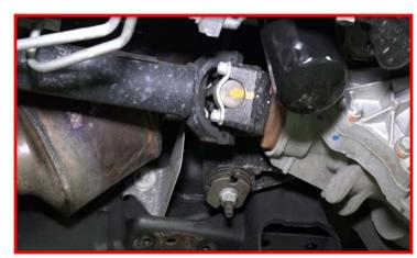
Disconnect the electrical connector at the passenger side differential actuator. Remove the harness from the differential. Remove the rubber diff vent hose from the diff.
