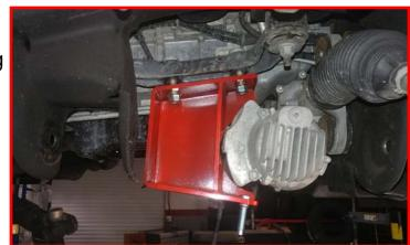
Install the ReadyLIFT driver side differential bracket to the factory hanger using the factory hardware. Do not tighten at this time.
