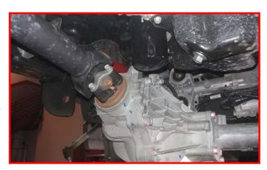
Install the ReadyLIFT rear cross member using the factory hardware from the outside facing inwards towards the differential. Do not tighten at this time.
