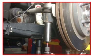
Remove the wire harness clips from the strut studs. Remove the upper strut hardware from the frame.
