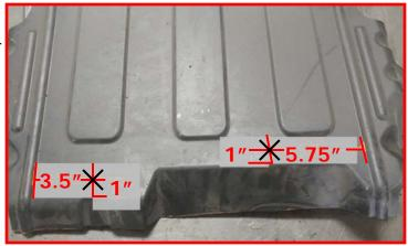
Flip the gravel guard over so that you are looking at the engine side. Locate the ReadyLIFT gravel guard brackets. The long one is the driver side and short is the passenger side. Install using the provided 3/8" x 1" bolts, washers, and lock nuts. Tighten so that the brackets are snug but still able to slightly pivot.
