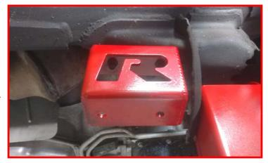
Install the sway bar to the ReadyLIFT brackets using the provided M10 x 40mm bolts, washers and locking nuts. Torque to 35 ft-lbs.
