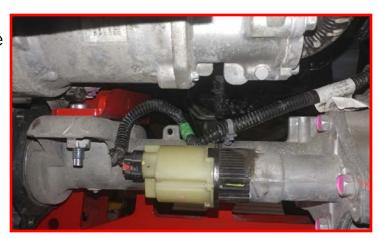
Locate the front gravel guard. Measure from the back edge towards the front 17.75".
