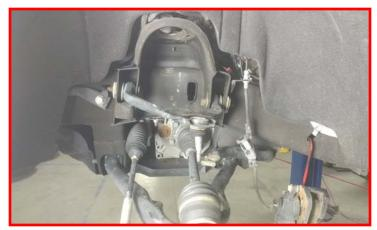
Remove the CV axle from the differential.
