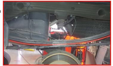
Install the ReadyLIFT block making sure the tapered end goes to the front of the vehicle. Raise the axle while lining up the center pins on the axle and block. Install the provided u-bolts. Do not fully tighten at this time. Repeat for the other side of the vehicle.
