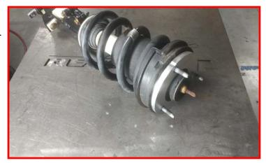
Install the completed strut assembly to the vehicle frame using the factory hardware. Do not tighten at this time.
