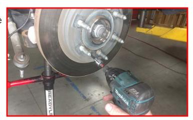
Remove the axle nut cover if installed. Remove the axle nut.
