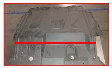
Measure out from the long inside rib on the driver side 5.75" and on the passenger side 3.5" and draw a parallel line with the rib. Measure from the lower edges on the driver and passenger sides up 1" and draw a parallel line with the edge. Where your lines intersect, use a 3/8" drill bit and drill a hole.
