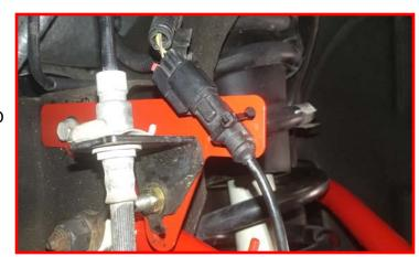
Locate the metal brake line bracket in the middle of the rubber line. Use a suitable cutting tool (cut off disk shown) cut a scribe line into the bracket. DO NOT cut through the metal into the rubber line. Once the line has been cut, you can bend the bracket open and remove from the rubber line. Once removed, zip tie the ABS wire to the rubber line.
