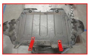
Install the assembled gravel guard to the core support cross member and front cross member using the factory hardware. The ReadyLIFT brackets will line up with the two original holes of the gravel guard. Hand tighten these only as they are self tapped holes and can strip easily.
