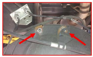
Install the ReadyLIFT brake line and ABS brackets to the axle using the factory hardware. Torque to 5 ft-lbs. The brake line bracket has a slight bend and will lean towards the front of the truck when installed properly.
