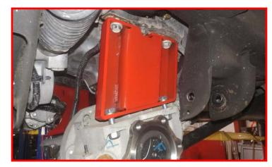
Install the differential to the passenger side ReadyLIFT bracket using the provided M12 x 45mm bolt, washer and factory nut to the rear most hole, and the factory nut to the stud on the bracket. Do not tighten at this time.
