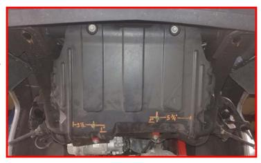
Install the ReadyLIFT front cross member to the frame using the factory hardware. Do not tighten at this time.
