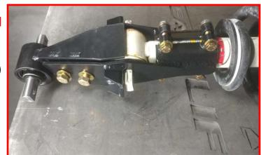
Install the strut cross bar to the Ready-LIFT clamshell using the provided 3/8" x 1.25" bolts, washers and locking nuts. Torque to 35 ft-lbs.
