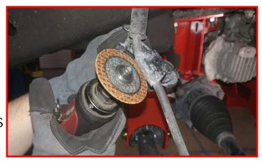
Magna ride vehicles: Take the removed brake line bracket and place in a vice. Mark as shown and cut the clamp side off. Bolt to the upper control arm using the provided 1/4" nut or the factory hardware depending which arm you have. Torque to 5 ft-lbs. Reconnect the sensor linkage.
