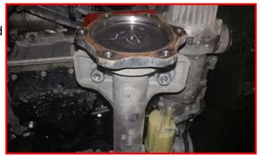
Install the front drive shaft to the pinion using the factory hardware and a drop of thread locker. Torque to 13 ft-lbs. Torque the differential hardware to 45 ft-lbs in this order, driver upper, driver lower, passenger upper, and passenger lower. While tightening the pass lower, center the bracket in the slotted holes.
