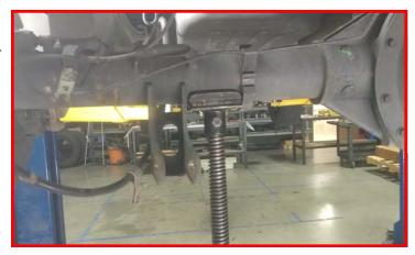
Loosen but do not remove the u-bolts on the opposite you are working on. Completely remove the u-bolts on the side you are working on. Lower the axle enough to remove the factory block.
