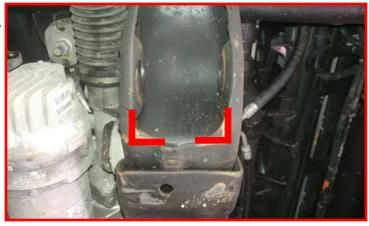
Install the ReadyLIFT passenger side differential bracket to the frame mount using the provided M12 Locking nuts and washers. Do not tighten at this time.
