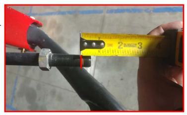
Hold the outer tie rod end in a vice. Measure from the end 1/2" and make a mark. Use a suitable cutting tool and cut off the end. Sand any burs off the end. Install onto the already cut inner tie rod end.
