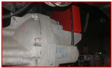
Re-connect the electrical connector on the differential actuator. Make sure to push in the safety lock. Zip tie the harness to the locating holes on the differential housing at the first and second mounts. Leave the one closest to the drive side undone.
