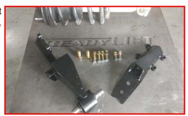
Install the ReadyLIFT clamshell mount around the lower strut body. Make sure to mount the clamshell to the strut with the inside angle towards the frame side of the strut.
