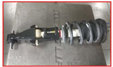
Bolt the two halves together using the provided 1/2" x 1" bolts and washers. Do not tighten at this time.
