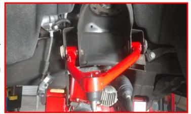
Late 2016 and newer vehicles with stamped steel arms: Locate the front upper control arm drop limiter. Remove the rubber isolator from the frame.
