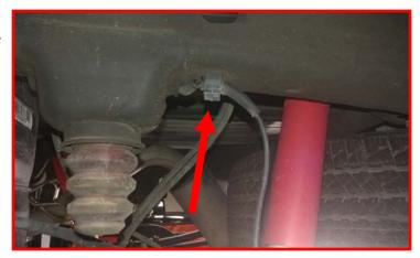
Route the driver side electrical connector to the inside of the frame rail. Disconnect the electrical connection. Let the driver side ABS wire hang free.
