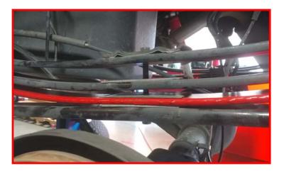
Use the clamp from the previous step and suck the leaf pack together. Do not use the center pin to suck the leaf's together. Once tight, cut the excess pin off above the nut.
