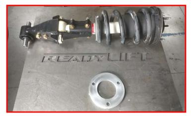
Install to the completed strut assembly with the large end of the taper to the outside of the vehicle. The shim has a locating notch to indicate outside. It will only fit on the strut one way.
