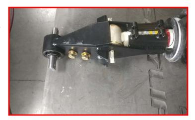
Install the 3/8" x 1.75" bolts, washers and locking nuts. Torque the 1/2" hardware to 45 ft-lbs, and the 3/8" hardware (using a criss cross pattern between the two sides) to 35 ft-lbs.
