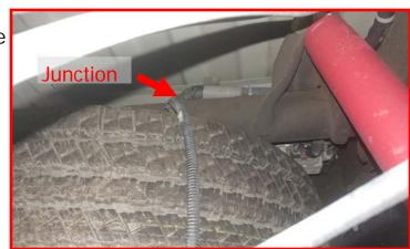
Locate the parking brake cable bracket on the driver side shock mount. Remove from the axle.
