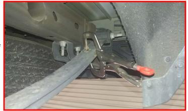
Use a suitable clamp at the leaf pack near the center pin. Remove the center pin. A pair of vice grips may aide in the removal of the pin to keep it from spinning. Once removed, release the clamp while supporting the overload spring.
