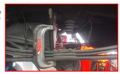
The overload spring will have a roll pin as a locater for when the spring pack was assembled at the factory. This needs to be removed. Use a suitable punch and tap the roll pin out of the leaf.
