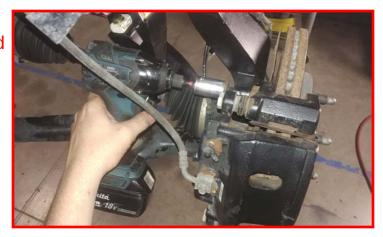
Install the ReadyLIFT brake line bracket to the frame rail using the factory hardware. Hand tighten only as this is a self tapped hole and can strip easily. Gently pull down on the metal line and install the bracket to the ReadyLIFT bracket using the provided 5/16" x .75" bolts, washers and locking nuts. Torque to 5 ft-lbs.
