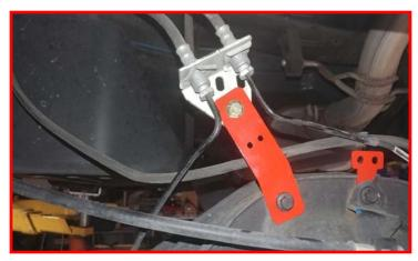
Connect the ABS electrical connector. Make sure to push in the safety clip. Route the ABS harness and vent tube along the rubber brake lines using zip ties. There are two holes in the ReadyLIFT brake line bracket for a zip tie as well.
