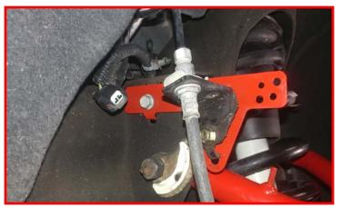
Route the ABS wire under the tie rod end boss on the knuckle and over the CV axle.
