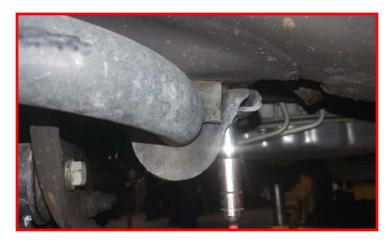
Remove the gravel guard from the frame.
