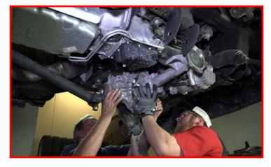
Locate the front control arm pockets. Mark the shown area. Use a suitable cutting tool, notch the corners of the pocket. (2wd: Necessary!)
