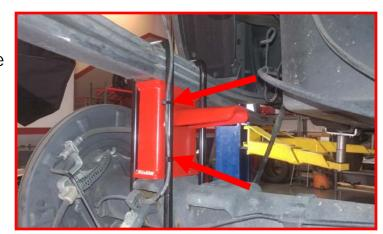
Driver side: Connect the ABS electrical connector at the frame rail. Make sure to push in the safety clip. Reposition the frame clip around the ABS wire.
