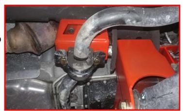
Install the factory sway bar end links to the lower control arm and sway bar. Tighten until there is a "1/4" squish on the rubber bushings.
