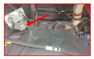
Remove the brake line bracket from the axle and discard. Remove the parking brake from the axle.
