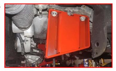
Support the differential, raise and install the differential to the driver side Ready-LIFT mount using the provided M12 x 45mm bolts, washers, and locking nuts. Do not tighten at this time.
