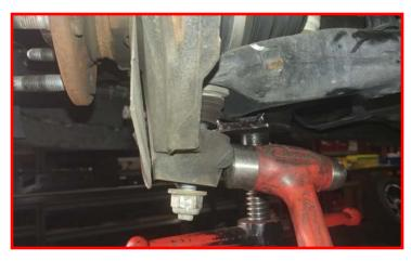
Remove the knuckle from the vehicle.
