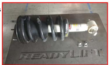
Locate the ReadyLIFT front clamshell strut extensions and hardware. (1/2" x 1" bolts, washers, 3/8" x 1.25" bolts, 3/8" x 1.75" bolts, washers and locking nuts) You will see the clamshell is angled. This angle is important to driver and passenger side. Passenger side shown.
