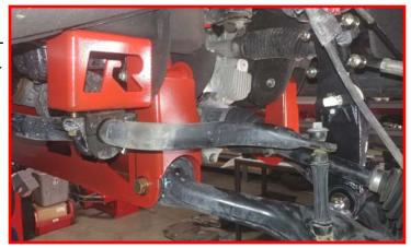
Locate the front differential assembly tab. Mark a line across the tab as shown.
