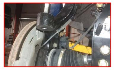
Connect the electrical connectors making sure to push in the safety clip. Clip the ABS connecter to the ReadyLIFT bracket. There are two holes for the clip. Use a zip tie through the remaining holes to secure the electrical connector to the bracket.
