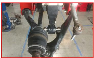
Locate the ReadyLIFT CV axle spacer. Note the chamfered side.
