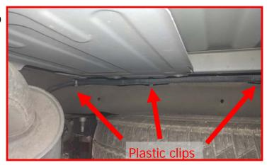
The harness will come to a junction on the rear cross member. Remove from the frame rail to this point. Let harness hang out of the way.
