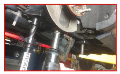
Strike the ball joint boss with a dead blow hammer to dislodge the taper.
