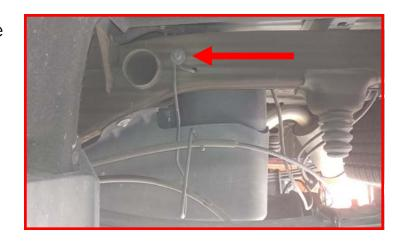
Take the passenger side parking brake cable and route it into the factory hanger to the lowest loop. Do not install the driver side parking brake cable. Install the factory hanger to the frame rail using the factory hardware. Hand tighten only as this is a self tapped bolt hole and can strip easily.
