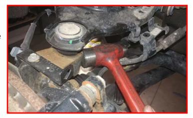
Loosen but do not remove the lower ball joint nut.
