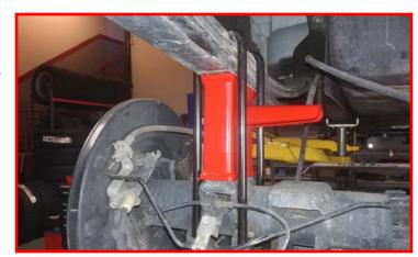
Install the provided shocks using the factory hardware. Do not tighten at this time.
