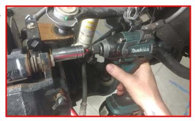
Use a suitable device, hang the caliper out of the way. Do not let the caliper hang by the rubber line.
