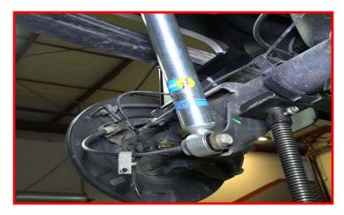
Gently bend the metal brake line upwards and attach the ReadyLIFT bracket using the provided 5/16" x .75" bolt, washers and locking nuts. Torque to 5 ft-lbs.
