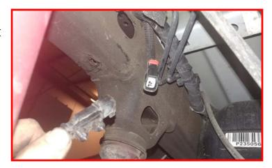
The passenger ABS harness is clipped into the rear cross member and frame rail. Remove the harness from the frame.
