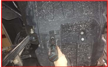
Remove the factory rear cross member from the frame. (2wd: Loosen but removal is not necessary)
