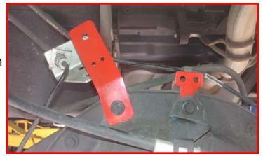
Clip the electrical connector into the ReadyLIFT ABS bracket. Route the passenger side ABS wire along the passenger metal brake line using zip ties.
