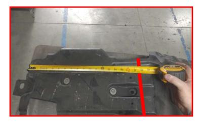
Mark a straight line across the gravel guard. Use a suitable cutting tool, cut along the line. Discard the lower half. Sand any burs off the cut edge of the front half.
