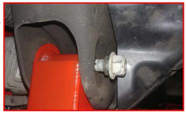
Install the lower control arms using the provided 5/8" x 4.5" bolts, washers and locking nuts in the forward mount and the provided 5/8" x 5.5" bolts, washers and locking nuts in the rear mount. Do not tighten at this time. Torque the cross member to frame hardware to 150 ft-lbs. (2wd: torque factory cross member to 45 ft-lbs)
