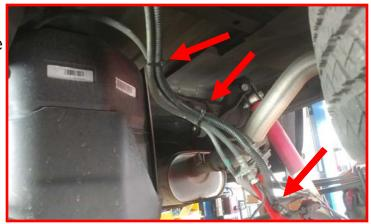
Driver side: Route the drive ABS wire up beside the ReadyLIFT block. Zip tie to the u-bolt.
