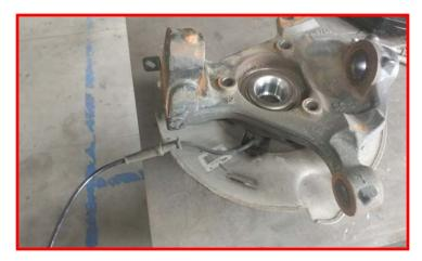
Install the ReadyLIFT knuckle using the factory hardware and a drop of thread locker. Torque to 55 ft-lbs.
