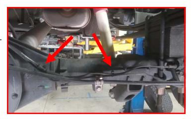
Support the axle with a suitable jack. Remove the shocks from the frame and axle.
