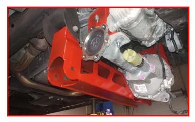
Make sure to reuse the factory tapered washer that was under the nut. Make sure to install with the taper towards the frame rail. Do not tighten at this time.
