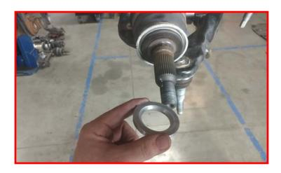
Install onto the CV axle with the chamfered side towards the axle.
