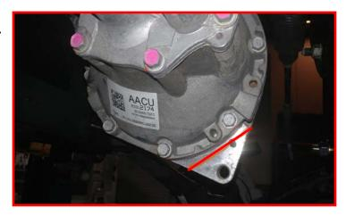
Use a suitable cutting tool, cut off the protruding mount. Sand all burs.
