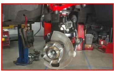
Drop the outer tie rod into the knuckle. Loosen the jam nut and remove the outer tie rod end.
