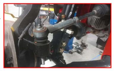
Measure from the end of the inner tie rod 1/2" and make a mark. Use a suitable cutting tool and cut off the end. Sand any burs off the end. Coat the end with antiseize.
