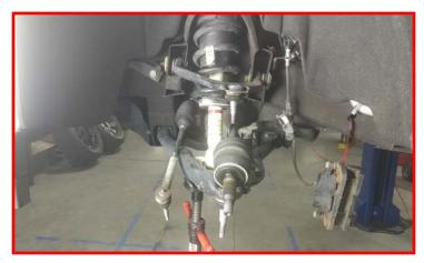
Remove the lower strut mounting hardware from the lower control arm.
