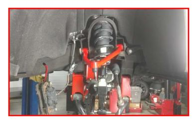
Raise the lower control arm up to the strut cross pin. Install the cross pin to the lower control arm using the provided M10 x 60mm bolts, washers and locking nuts. Torque to 45 ft-lbs.
