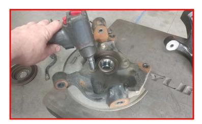
Remove the ABS wire from the bracket. Discard the plastic clip.
