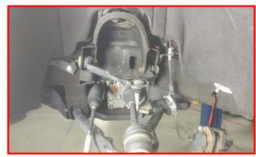
Remove the CV axle from the differential.
