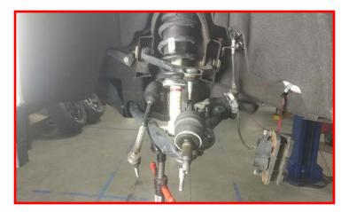
Remove the lower strut mounting hardware from the lower control arm.
