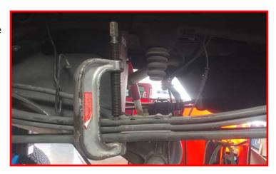
The overload spring will have a roll pin as a locater for when the spring pack was assembled at the factory. This needs to be removed. Use a suitable punch and tap the roll pin out of the leaf.
