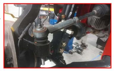
Measure from the end of the inner tie rod 1/2" and make a mark. Use a suitable cutting tool and cut off the end. Sand any burs off the end. Coat the end with antiseize.
