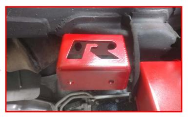
Install the sway bar to the ReadyLIFT brackets using the provided M10 x 40mm bolts, washers and locking nuts. Torque to 35 ft-lbs.
