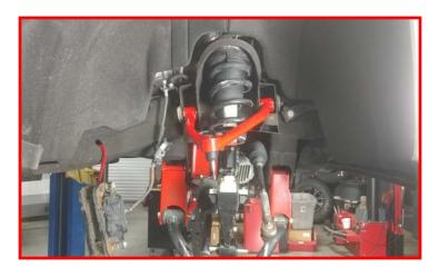
Raise the lower control arm up to the strut cross pin. Install the cross pin to the lower control arm using the provided M10 x 60mm bolts, washers and locking nuts. Torque to 45 ft-lbs.
