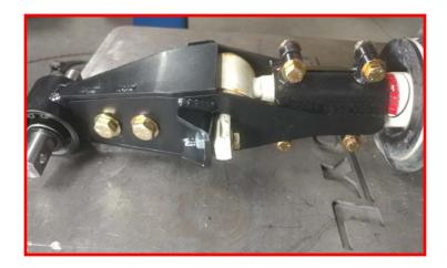
Locate the ReadyLIFT tapered strut shim.
