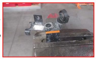
Locate the ReadyLIFT sway bar brackets. There is a left and right side specific. The mounting holes are offset to the front on the upper mount and to the rear on the lower. This locates the sway bar to the rear of the vehicle. Install using the factory hardware. Torque to 35 ft-lbs.
