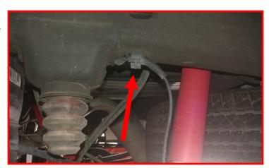
Route the driver side electrical connector to the inside of the frame rail. Disconnect the electrical connection. Let the driver side ABS wire hang free.
