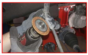
Magna ride vehicles: Take the removed brake line bracket and place in a vice. Mark as shown and cut the clamp side off. Bolt to the upper control arm using the provided 1/4" nut or the factory hardware depending which arm you have. Torque to 5 ft-lbs. Reconnect the sensor linkage.
