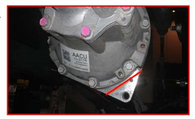
Use a suitable cutting tool, cut off the protruding mount. Sand all burs.
