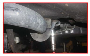
Remove the gravel guard from the frame.
