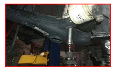
Remove the strut from the vehicle.
