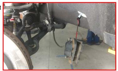
Remove the rotor from the knuckle. Some rotors are held on by a torx bolt and this must be removed. Set aside.
