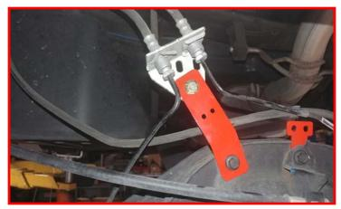
Connect the ABS electrical connector. Make sure to push in the safety clip. Route the ABS harness and vent tube along the rubber brake lines using zip ties. There are two holes in the ReadyLIFT brake line bracket for a zip tie as well.
