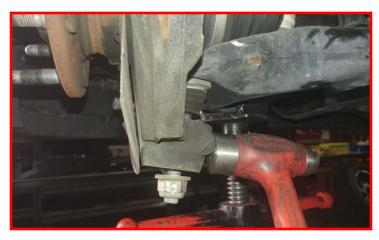
Remove the knuckle from the vehicle.
