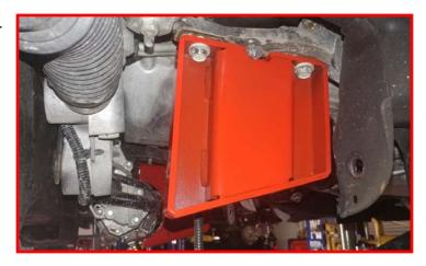
Support the differential, raise and install the differential to the driver side Ready-LIFT mount using the provided M12 x 45mm bolts, washers, and locking nuts. Do not tighten at this time.
