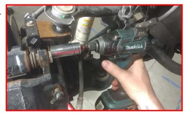
Use a suitable device, hang the caliper out of the way. Do not let the caliper hang by the rubber line.
