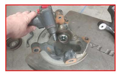
Remove the ABS wire from the bracket. Discard the plastic clip.
