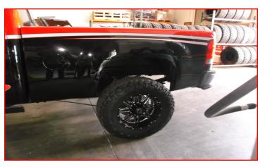
Move to the front of the truck. Set the ride height of the vehicle by measuring from the center of the wheel to the fender edge straight above. Make sure that if you have deep dish wheels, that you use a straight edge and level to find center of the wheel and straight edge at the fender. DO NOT measure by going around the lip of the wheel. Use of a straight edge and level may be necessary for deep dish wheels.
