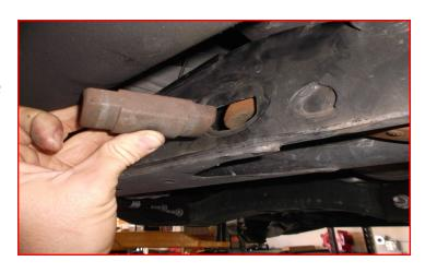
Mark the torsion bar end for reassembly. It is very important that they go back into the vehicle the way they came out. Slide the torsion bar forward through the lower control arms while holding onto the keyways. Remove the keyways from the cross member. Let the torsion bars hang from the lower control arm.
