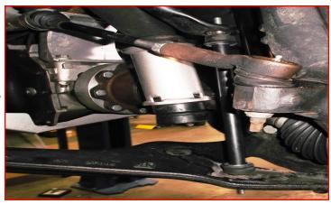
Install your extended length shocks to the frame using the hardware that either came with the shocks or the factory hardware. Install the lower shock mount to the lower control arm using the factory hardware. Torque to 60 ft-lbs.
