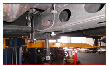
Add pressure by tightening the forcing screw to the torsion bar until there is enough room to remove the torsion bar adjustment pin from the cross member. Once the pin is removed, release the pressure on the torsion bar by loosening the forcing screw. Repeat for both sides.
