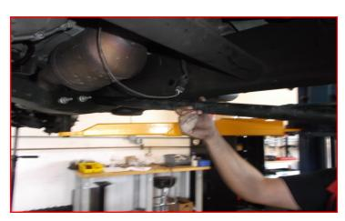
Remove the sway bar end links from the sway bar and lower control arm. Make sure to save all the rubber ends. If they are worn or bad, replace with new. You will have to remove the capture nut and any washers inside the rubber ends. They will be replaced.
