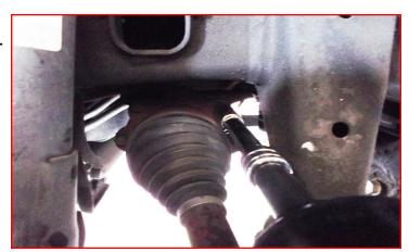
Remove the CV axle from the vehicle.
