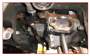
Clean the driver side rear control arm pocket. Measure from the center of the control arm mounting bolt to the inside of the frame pocket 1.25", mark a line vertically across the back and front side of the pocket. Connect the two lines across the top of the pocket.
