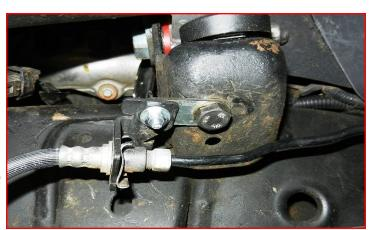
Install the outer tie rod ends to the ReadyLIFT knuckles using the factory hardware. Torque to 65 ft-lbs.
