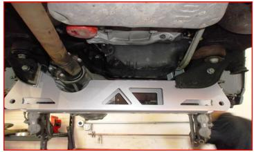
Install the ReadyLIFT front cross member using the factory control arm hardware. Do not tighten at this time.
