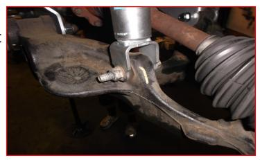
Install the ReadyLIFT sway bar end links to the lower control arm and sway bar using the factory rubber isolators, provided M10 fender washers and M10 nuts. Torque to 15 ft-lbs.
