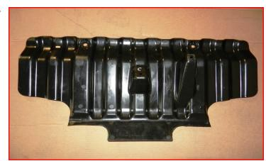
Install the gravel guard between the ReadyLIFT cross member and the factory cross member. As you raise the guard to the core support bar, make sure to guide the lower radiator hose clamp into the guard mounting hole. Press into place. Install the front edge to the factory core support bar using the factory hardware. Tighten down by hand.
