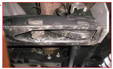
Install the ReadyLIFT front skid pate using the provided 3/8" bolts and washers. Torque to 30 ft-lbs. Torque the front and rear cross member to frame hardware to 150 ft-lbs.
