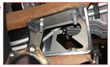
Install the ReadyLIFT driver side diff drop to the original hanger using provided M12 bolts and washers to the forward two locations. Install the last mount using the factory bolt and a provided M12 washer and nut. Install the differential to the ReadyLIFT bracket using the factory bolts in their proper location and provided
