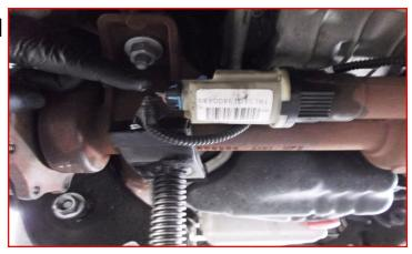
Mark the front drive shaft to pinion orientation for reinstallation later. Remove the front drive shaft from the differential. Let hang out of the way.
