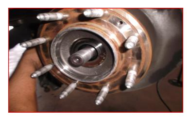
Remove the hub bearing mounting hardware from the knuckle. Make sure to not drop the hub assembly. Remove the dust shield with the assembly.
