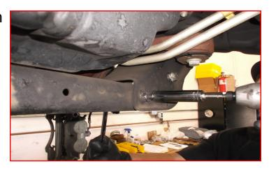
Remove the electrical connectors and vent tube from the differential.
