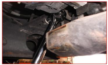
Once the cross member is removed, pull the torsion bars out of the lower control arms and set aside. Make sure to have the bars marked for reassembly. It is best to lay the bars down on the ground under the vehicle in the same orientation/side as they are removed.
