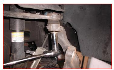
Mark the CV axle flange to the differential flange and driver / passenger side for reinstallation later. Remove the CV axle hardware.
