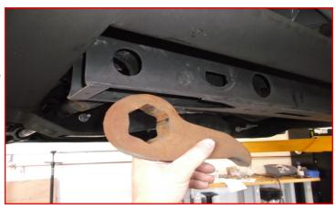
With the torsion bar slid forward, remove any wire harness that is attached to the cross member. Remove the torsion bar cross member from the frame.
