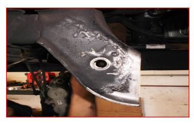
Check your front lower control arm pockets. If there is any material hanging below the frame rail from the control arm pocket, use a suitable cutting device and notch the painted section flush with the frame rail weld. Do not cut the weld off the pocket. If your truck does not have this piece hanging under, ignore.
