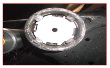
Install the ReadyLIFT bump stop extension using provided 3/8" x 5.5" long Allen head bolt and washer. Torque to 35 ft-lbs.
