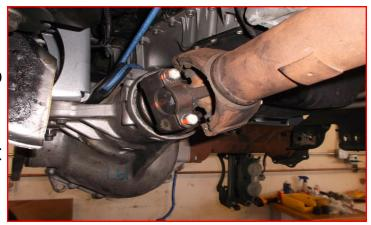
Install the ReadyLIFT rear cross member using the factory control arm and cross member hardware. Do not tighten at this time.
