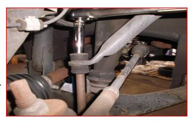
Remove the outer tie rod end hardware. Strike the tie rod boss on the knuckle with a dead blow hammer to dislodge the taper.
