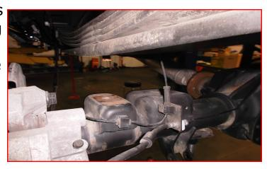
Install the provided u-bolts and nuts. Snug up but do not tighten at this time. Repeat for the opposite side. When tightening, use a criss-cross pattern. Alternate between sides of the vehicle.
