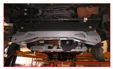
Install the lower control arms to the ReadyLIFT cross members using M18 bolts, washers, and nuts. Do not tighten at this time. If you are installing the 7-8" lift kit, Install the ReadyLIFT upper control arms now.
