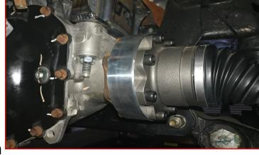
Install the ReadyLIFT passenger side CV (1" thick) spacer in between the CV flange and differential flange using the provided M10 x 50mm Allen bolts, washers and a drop of thread locker. Make sure to line up the previous marks on the flanges. Torque all CV bolts to 50 ft-lbs.
