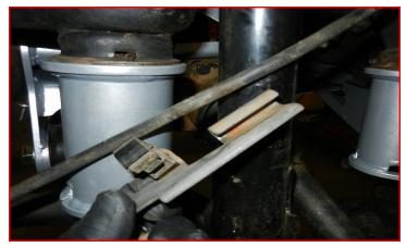
Install the ReadyLIFT brake line bracket to the frame using the factory hardware and to the factory brake line bracket using the provided 1/4" bolt, washers and nuts. Torque all to 5 ft-lbs. Reconnect the ABS electrical connection and install onto the frame rail. Run the ABS wire along and zip tie to the rubber brake line behind the knuckle.
