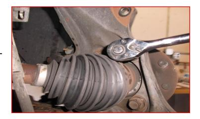
Loosen but do not remove the upper and lower ball joint nuts. Strike the ball joint boss on the knuckle to dislodge the tapers. Remove the knuckle from the upper and lower control arms.
