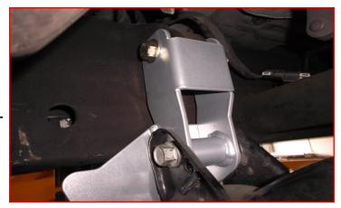
Install the torsion bars into the factory keyways for the 5-6" lift kit, and the ReadyLIFT keyways for the 7-8" lift. Using the torsion bar tool, load the torsion bar enough to install the cross pin and factory adjusting bolt. Set the adjustment bolt to the recorded lengths from the previous step for the initial setting.
