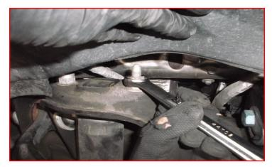
Take care when working with the torsion bars, as they are under extreme pressure and if handled incorrectly can cause injury and/or death. There are multiple styles of torsion bar tools available. Use the one that is correct for your year model range.
