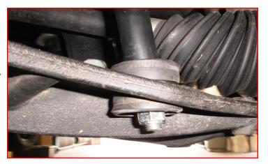
Install the torsion bars for the appropriate sides into the lower control arms and let hang. Make sure to install in the same orientation as previously removed or marked as in the prior steps for removal.
