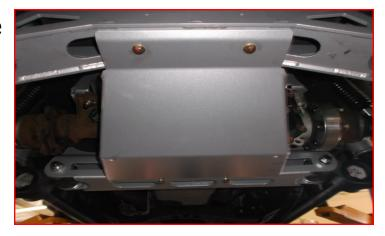
Trim the lower corners of the factory plastic gravel guard as shown. (You are removing the stepped area for the original lower bolts.)
