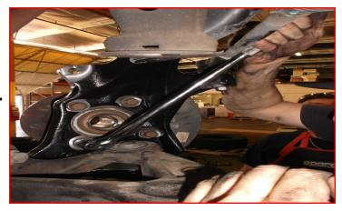
Install the CV axles to the hub assembly using the factory hardware. Torque to 200 ft-lbs. Install the ReadyLIFT driver side CV (1.5" thick) spacer in between the CV flange and differential flange using provided M10 x 60mm Allen bolts, washers and a drop of thread locker. Make sure to line up the previous marks on the flanges.
