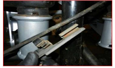
Install the ReadyLIFT brake line bracket to the frame using the factory hardware and to the factory brake line bracket using the provided 1/4" bolt, washers and nuts. Torque all to 5 ft-lbs. Reconnect the ABS electrical connection and install onto the frame rail. Run the ABS wire along and zip tie to the rubber brake line behind the knuckle.
