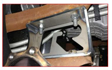
Install the ReadyLIFT driver side diff drop to the original hanger using provided M12 bolts and washers to the forward two locations. Install the last mount using the factory bolt and a provided M12 washer and nut. Install the differential to the ReadyLIFT bracket using the factory bolts in their proper location and provided
