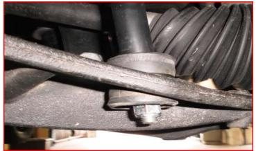
Install the torsion bars for the appropriate sides into the lower control arms and let hang. Make sure to install in the same orientation as previously removed or marked as in the prior steps for removal.
