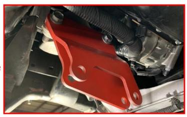
Install the passenger side front differential drop onto factory differential mounting point using the factory mounting bolts. Do not tighten at this time.
