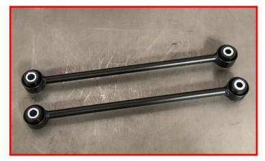
Install the completed sway bar end link assembly onto the frame using the supplied M10 x 70mm bolt and M10 fender washer. Do not tighten at this time.
