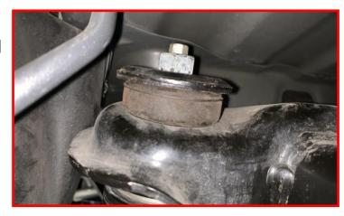
Loosen but do not remove the upper and lower trailing arm hardware.
