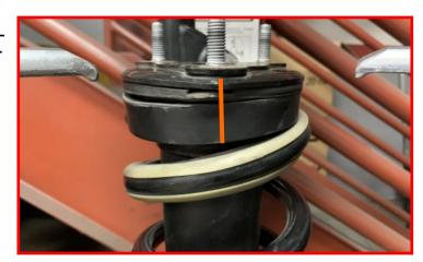
Install the ReadyLIFT preload spacer onto the dust shield/ spring seat. Install the factory top hat/rubber isolator on top of the preload spacer making sure to align the previous made marks. When tightening, make sure the top of the strut shaft is fully seated into the top hat.
