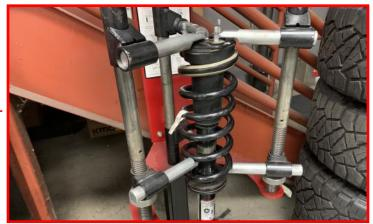
Mark the top hat to spring location for reassembly. Take care as the strut is under extreme pressure. Relieve the tension on the spring and remove the top hat.
