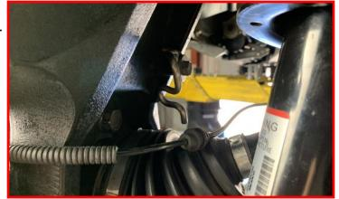
Install ABS sensor into knuckle using the factory hardware.
