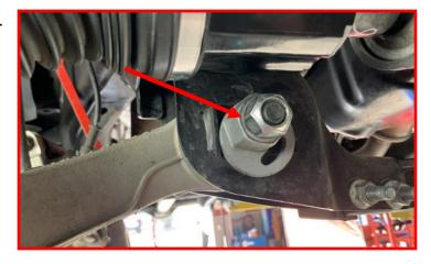
Remove the lower strut mounting bolts from the lower control arm. Retain factory bolts.
