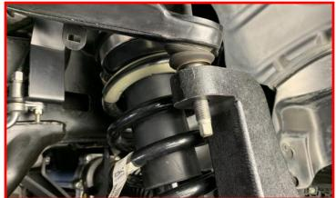
Install the opposite side ABS wire bracket on the inside of the knuckle using the factory hardware (i.e. Driver will be installed on passenger side).
