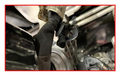
Remove the actuator harness retaining clip from the inside the frame rail.
