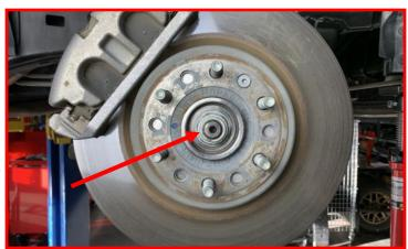
Remove brake caliper mounting bolts and hang caliper out of the way. Do not hang the caliper by the brake line. Retain factory hardware.
