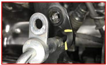
Remove brake line from factory mounting area.
