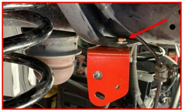
While gently pulling down on the brake line install the factory brake line bracket onto the driver rear brake line bracket using the factory hardware and supplied M8 nut and washer.
