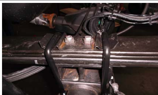
16. Be sure to locate the U-Bolts properly on top of Leaf Pack
