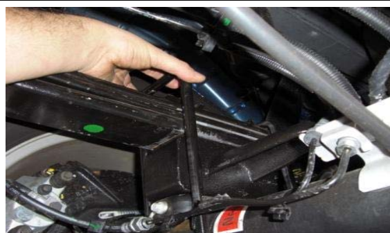
15. Replace u-bolts over leaf spring and axle.
