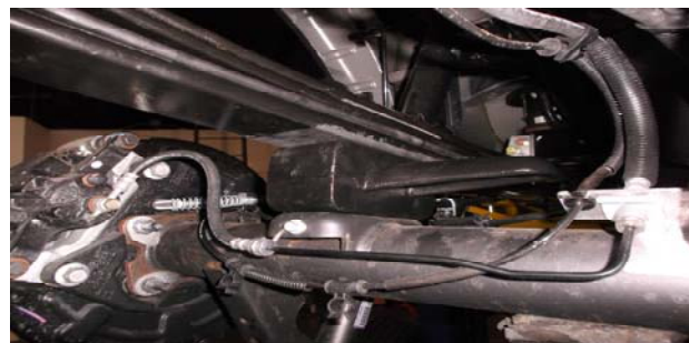
14. Raise axle up to engage lift block.
