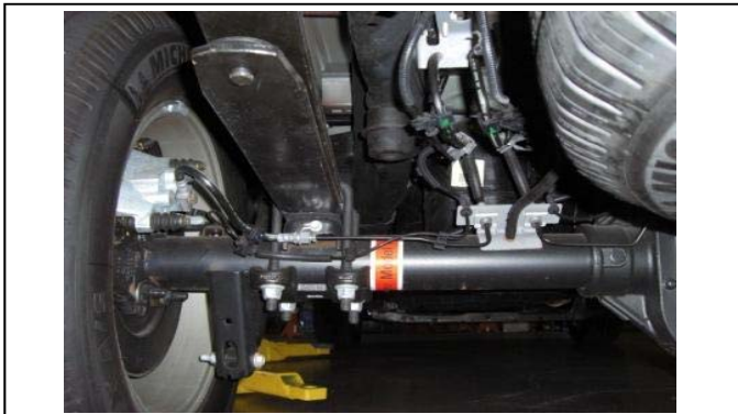
3. View of 2WD rear axle and leaf springs.
