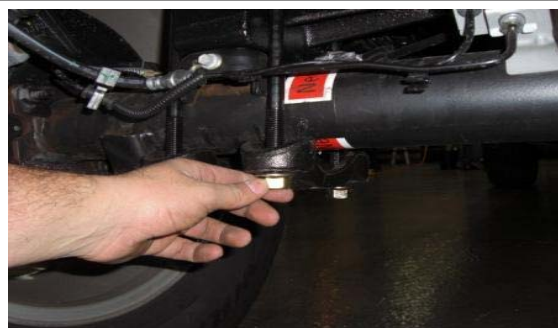
17. Replace lower spring plate and attach with nuts.
