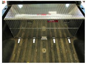
3) Drill one 5/16" hole in each tab and the bed of the truck (making sure as to not hit any wiring or other critical components of the truck) for mounting. Drill only one hole per tab. Place a bolt in your first hole to help keep the tank in-place while drilling the other holes.
