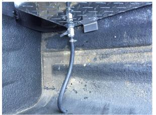
12) Measure the distance to the adapter and cut off the unneeded hose. Connect the hose to the control valve on top of the adapter and secure with a hose clamp.
