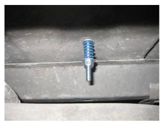
This spring bolt combination will anchor the tank while still allowing the tank to move with the bed of the truck as it travels over rough terrain. This will prevent undue stresses from being passed along to the tank from the truck.
