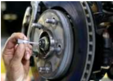
27. Your RCV CV joints can be greased using a needle tip grease adapter by inserting it into the zert fitting. **We recommend 3-4 pumps using a manual grease gun every 6 months.
