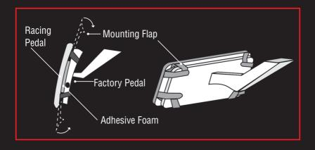
2. To install on the smaller size pedals, keep extra flaps not needed in their fold-in positions (Fig. 2)
