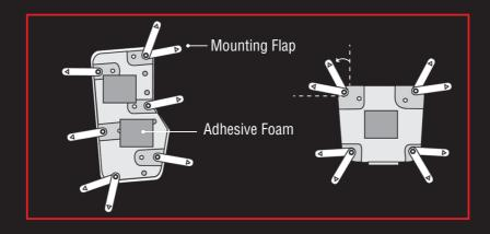
1. Rotate the mounting flaps on the rear side of the racing pedals, adjust each flap to a proper angle against the vertical/horizontal line, corresponding to the shape and the size of the factory pedal.
