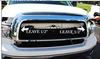
3. LAY NEW GRILLE IN OPENING OF GRILLE SHELL, PRESS GRILLE AGAINST SHELL AND SCREW THE SUPPLIED #8 SCREW THROUGH EACH OF THE 6 BRACKETS, THROUGH GRILLE SHELL, INTO SPRING NUTS. RE-ATTACH HOOD LATCH TO BRACKET ON NEW GRILLE.
