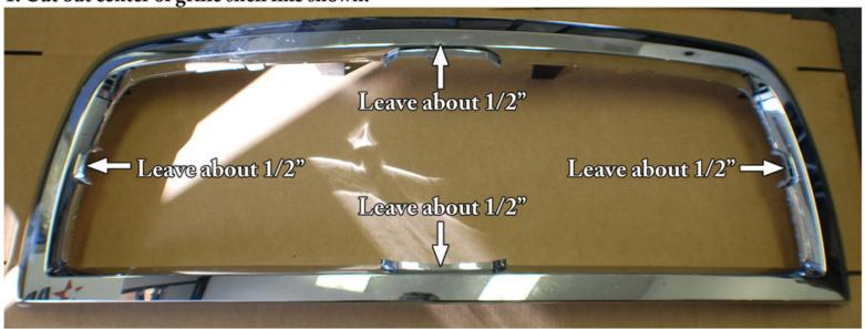
2. New grille comes with all the brackets attatched, Remove them and lay the new grille into the opening of the stock grille shell.
