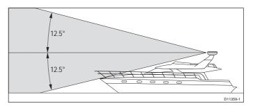
Mount the scanner so that the array rotates parallel to the waterline. The radar beam is approximately 25° wide in the vertical direction, giving good target detection when your boat pitches and rolls.
