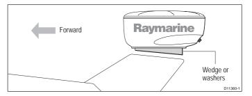
Planing hull and some displacement hull boats adopt a higher bow angle when the boat is at cruising speed, giving poor target detection. It may be necessary to lower the radar beam back towards the parallel, by shimming the rear of the radar, so that the beam points slightly down when the boat is at rest. Refer to the diagram on page 14 for more information.
