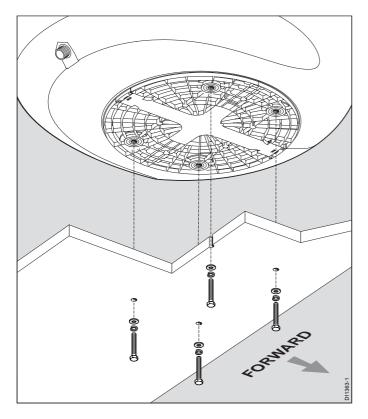
**Note:** The M8 bolts that secure the Digital Radome scanner to the mounting platform require a torque of 20Nm (177lbf.in). Use the supplied "Denso Paste" to lightly coat the mounting bolts.
