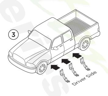
4. Align the Front, Center and Rear Driver's Side Brackets with
