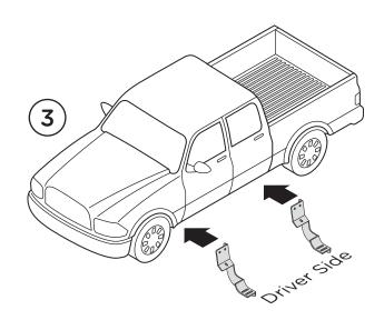
**4.** Align the Front and Rear Driver's Side Brackets with existing bolt and the existing hole located on the Rocker Panel.
